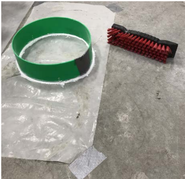
Figure 4-10: Scaling Resistance Mold Setup
