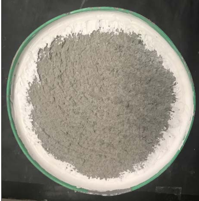
Figure 5-8: Before Conducting ASTM C672 PCCP 6 Rating = 0
