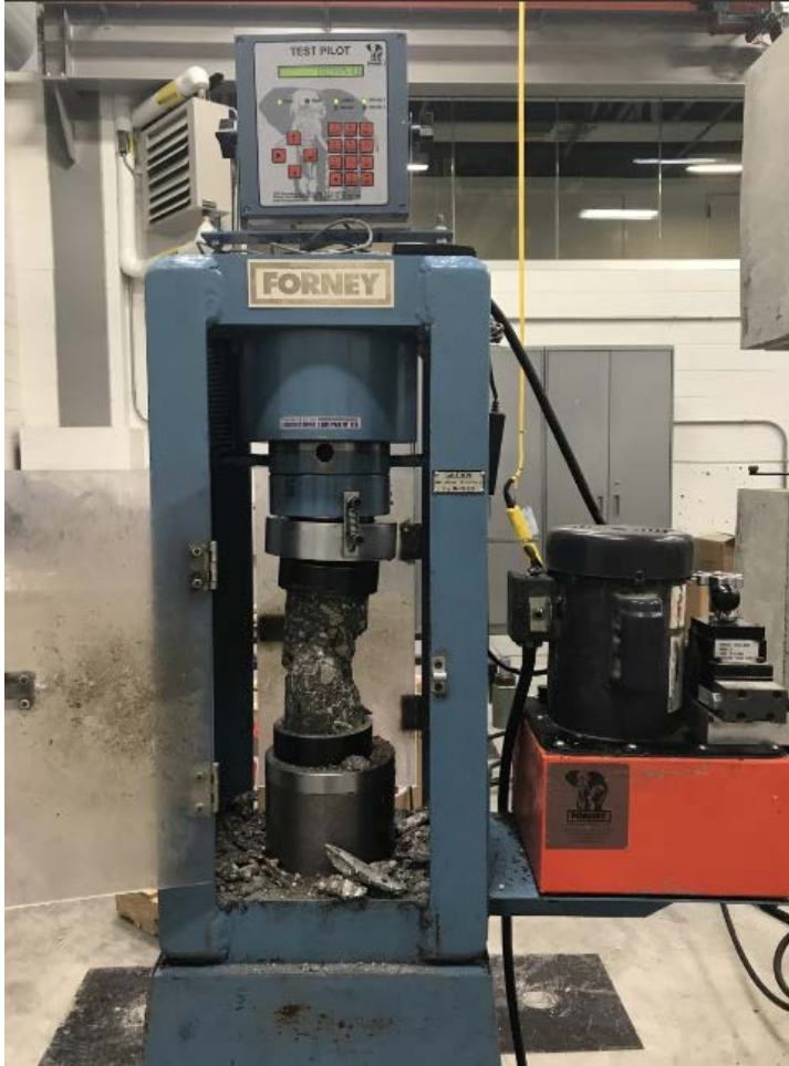
Figure 4-5: ASTM C39 Compressive Strength Test
