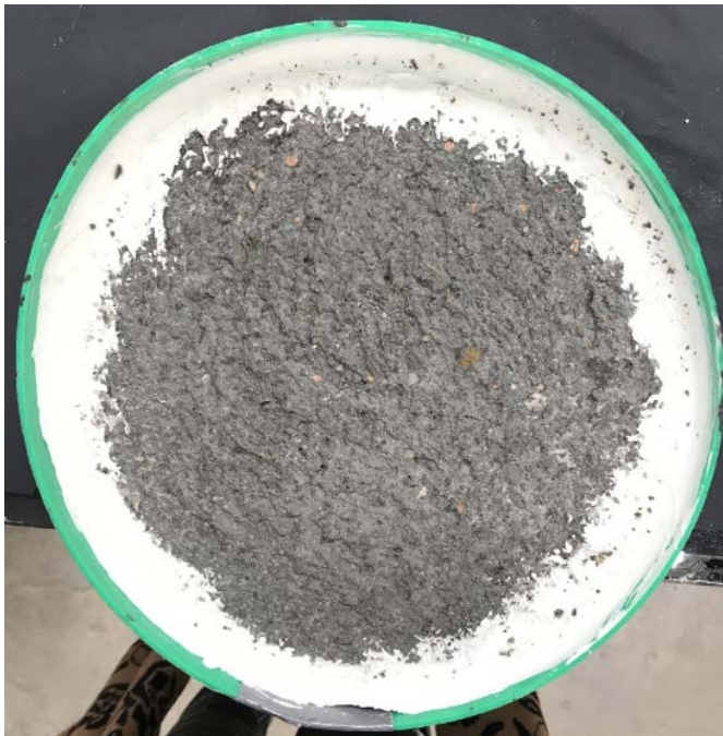
Figure 5-9: Before Conducting ASTM C672 PCCP 6 Rating = 2
