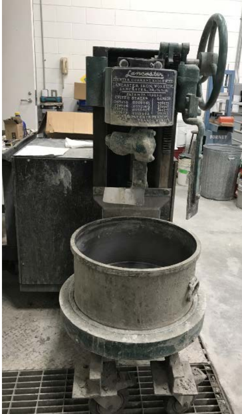
Figure 4-2: Lancaster Counter-Current Mixer
