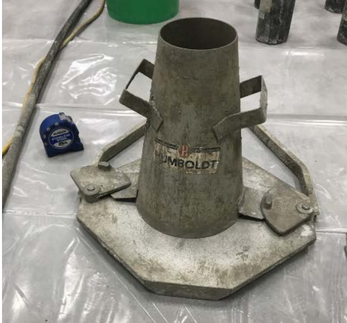
Figure 4-3: ASTM C143 Slump Test Equipment
