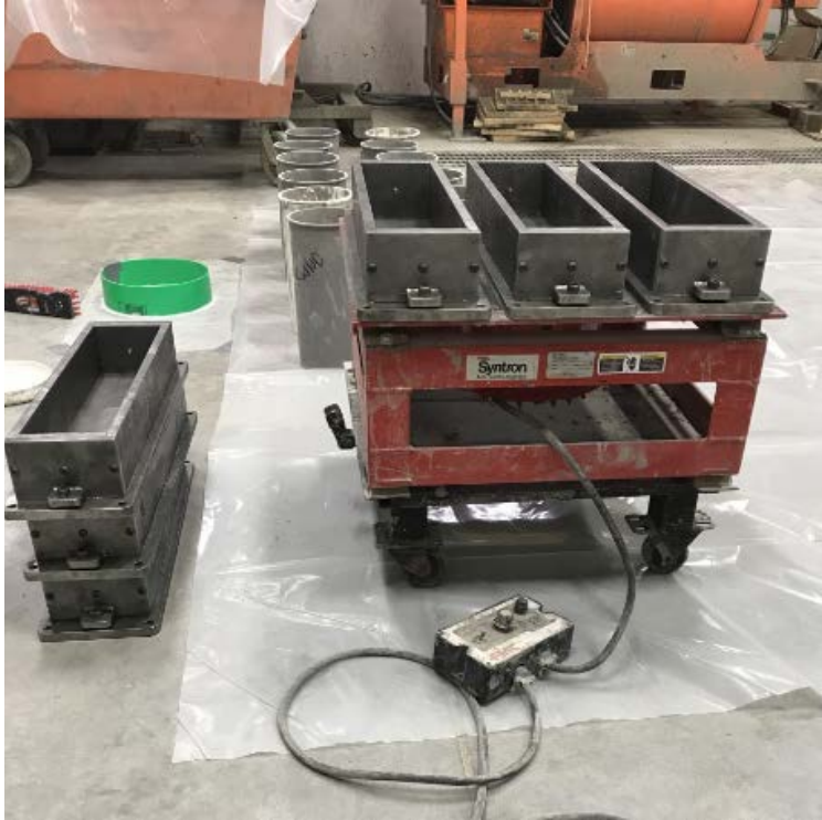
Figure 4-7: Setup for Casting Concrete Beams
