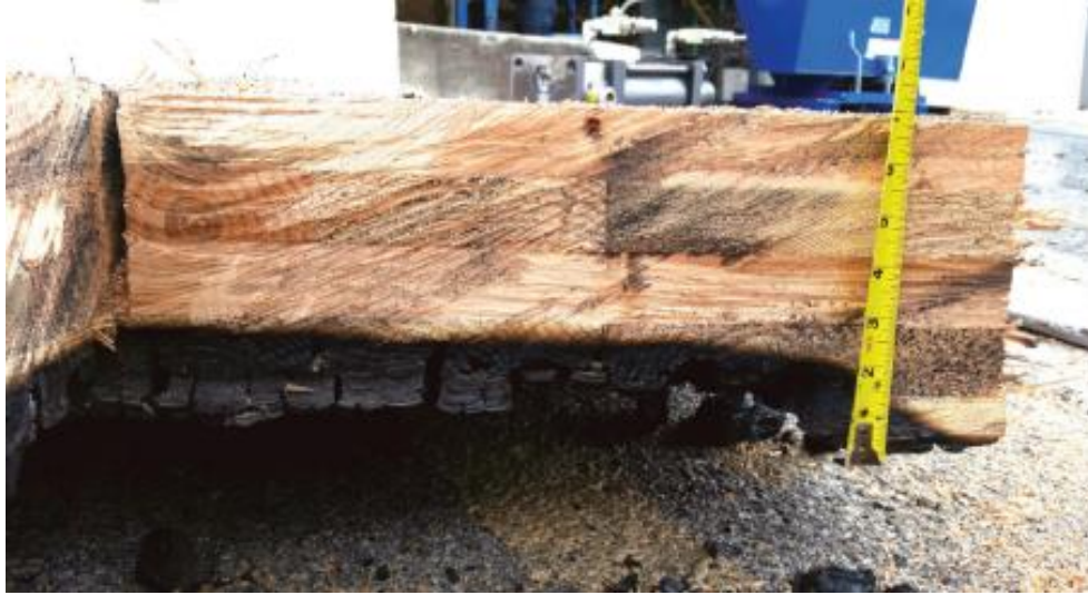
Figure 2.1. CLT Panel After Fire Test (Barber et al., 2022)
