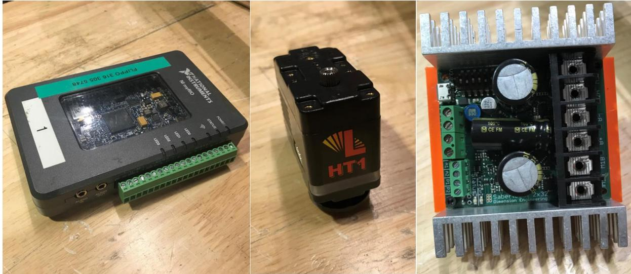
**Figure 12: MyRio (left), Servo Motor (center), Motor Controller (right)**
