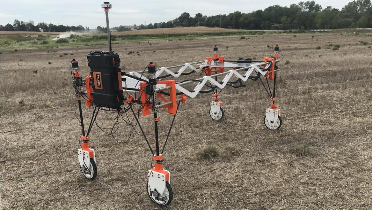
**Figure 14: Pancreas with Fiberglass Extended Frame**
