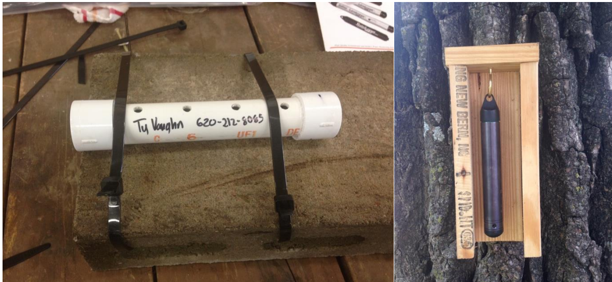
Figure 13: Pressure transducer vessels. The vessel on the left houses the Levelogger and the treehouse on the right houses the Barologger Edge.
