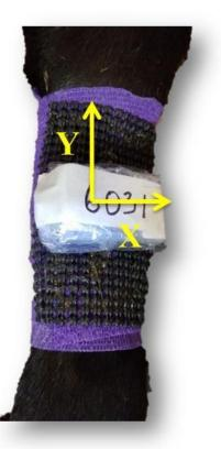
**Figure 2-7.** Accelerometer is placed with the purple side facing out (or numbered side) and the y-axis of the logger aligned with the leg.
