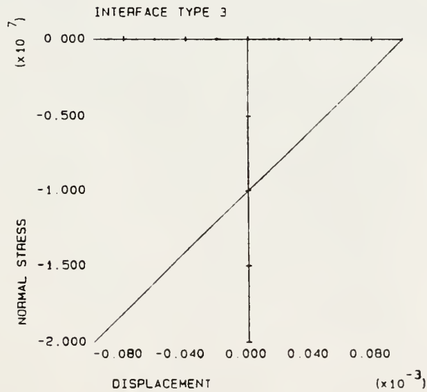
Figure 2.2: Typical Joint Opening Law Traction -- Displacement Relation
