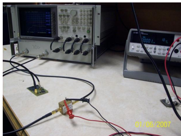
Figure 51: Test setup for ripple rejection plots.
