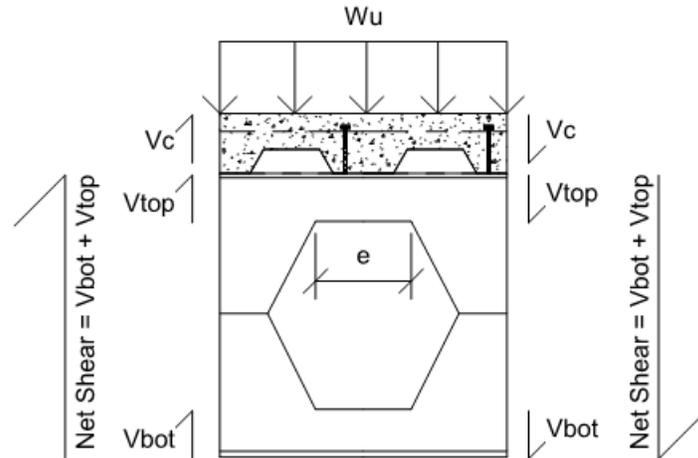
**Figure 3-10 – Composite Vierendeel Moment Derivation**
