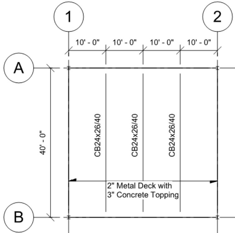
**Figure 4-7 – Composite Bay Floor Plan**
