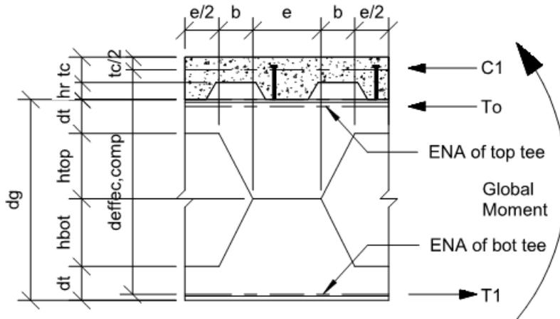
**Figure 3-9 – Composite Axial Forces**
