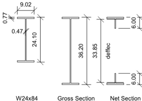
**Figure 4-3 – Beam Section Dimensions**
