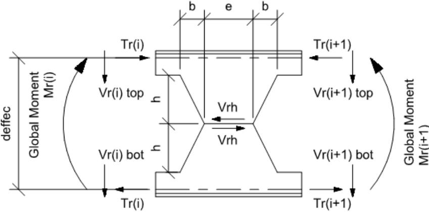
Figure 3-5 – Web Post Buckling Forces
