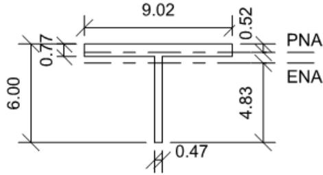
**Figure 4-5 – Tee Section Dimensions**
