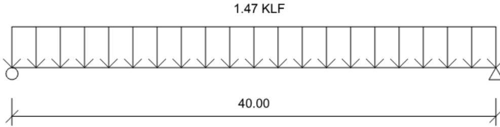
**Figure 4-8 – Beam Loading**
