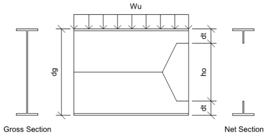
**Figure 3-7 – Vertical Shear Area**
