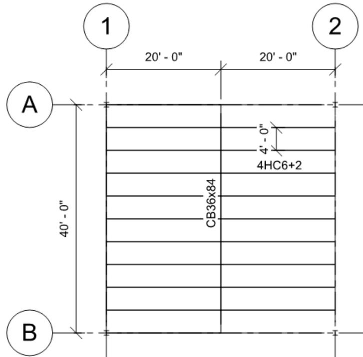
**Figure 4-1 – Bay Floor Plan
