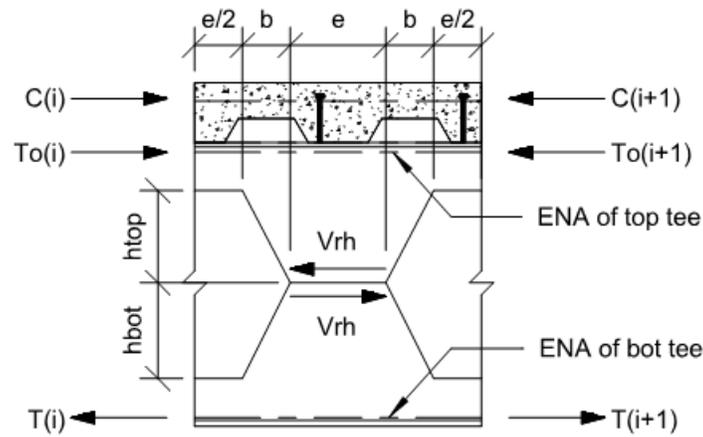
**Figure 3-11 – Composite Web Post Buckling Terms
