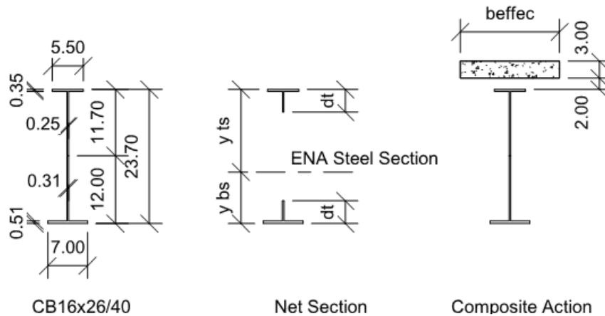
**Figure 4-9 – Composite Castellated Beam Section Dimensions**
