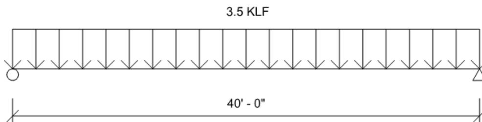
**Figure 4-2 – Beam Loading**
