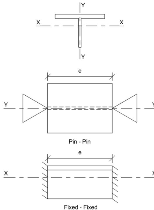
**Figure 3-2 – Tee Section Boundary Conditions**
