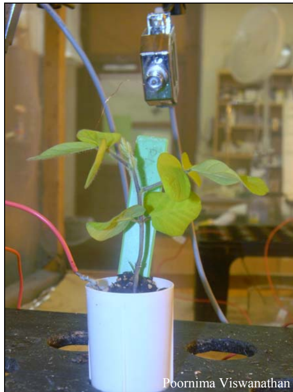
Figure 3.1. EPG set up showing plant electrode (V-2 stage plant) and insect electrode (wired aphid)
