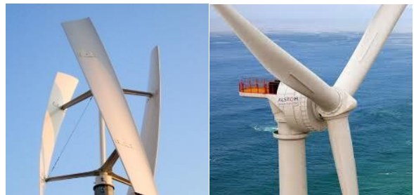
Figure 2.1 Horizontal (right) and vertical (left) axis wind turbine structures [56].
