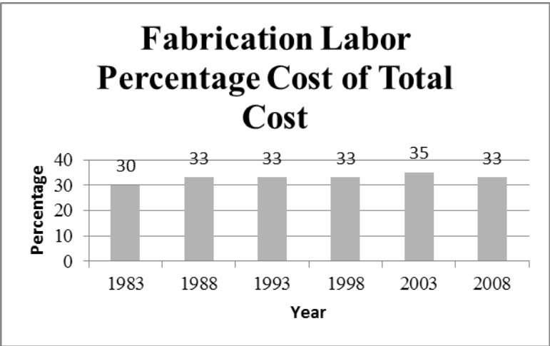
Figure 2-3: Fabrication Labor Percentage Cost (adapted from “$ave More Money” Modern Steel Construction March 2008)
