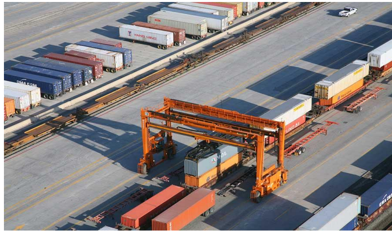
Figure 5-1 Intermodal terminal: unloading rail cars, loading chassis 1
