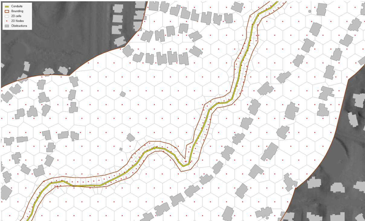
**Figure 4.4. The 2D mesh creation includes a boundary, 2D nodes, 2D cells, LiDAR, and obstructions layer.**
