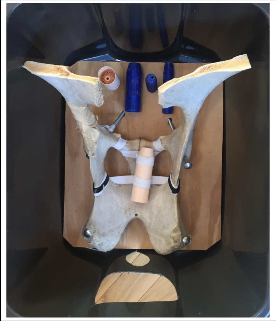
Figure E.4 - The 3D printed cervix assembled in the pelvic box from the top view
