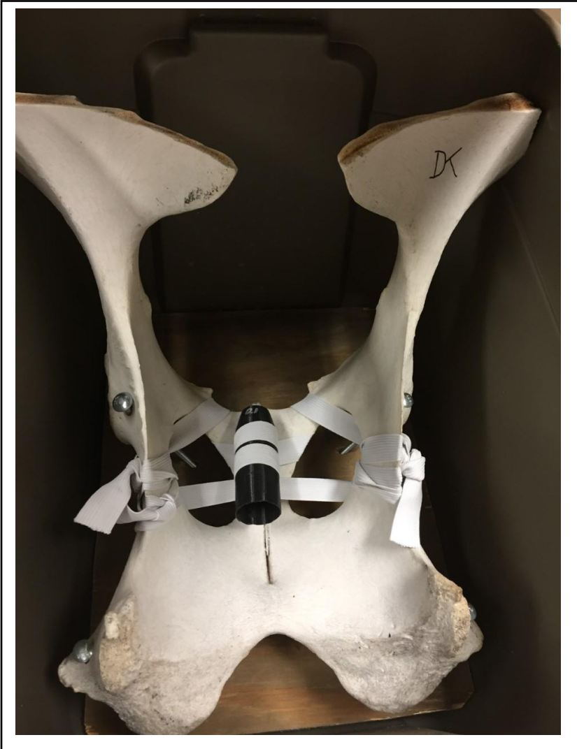
Figure E.5 - The 3D printed cervix assembled in the pelvic box from the rear view
