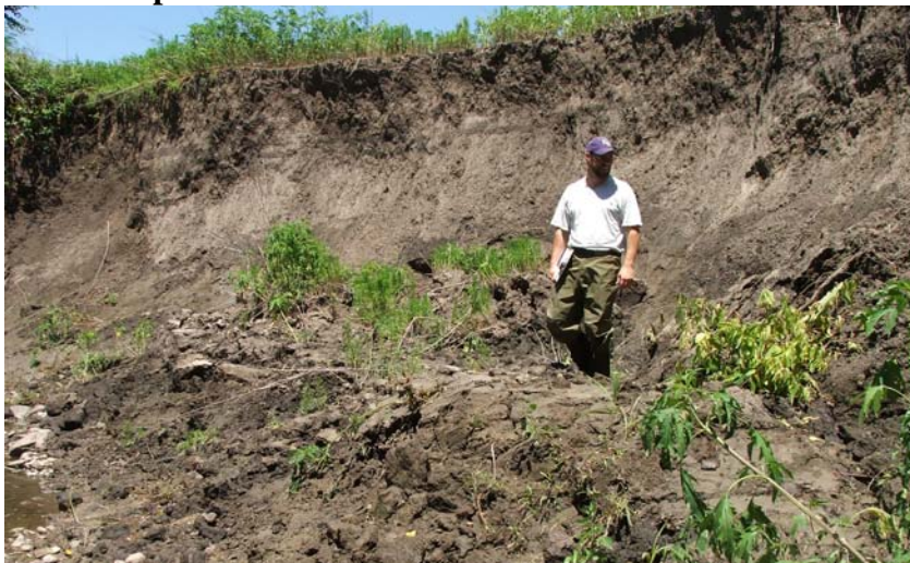
Figure 9. Irish Creek 2 Study Bank example illustrating loss of bank pins and toe pin. Bank slumped and left approximately one-third of the bank height at the bank toe; thus only 0.91m of retreat was assumed. The accompanying drawing illustrates the assumption of how the bank failed.
