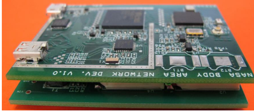
Figure 2-8: Combination of mother board and daughter board
