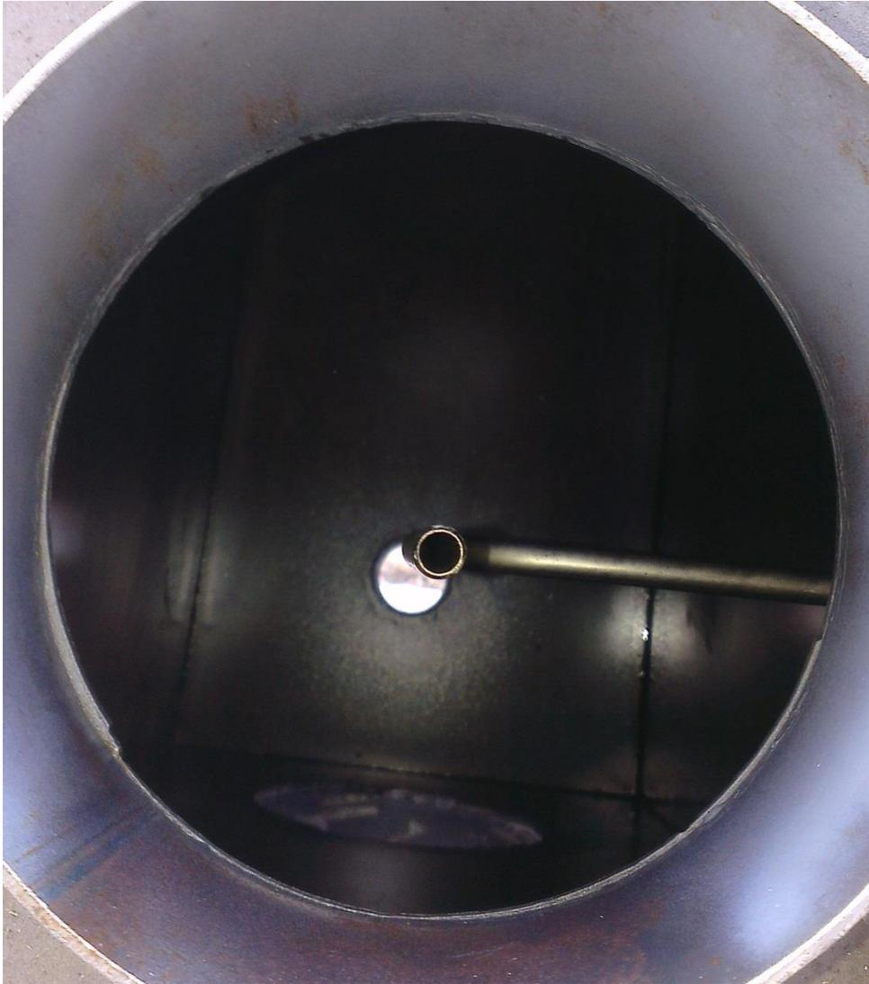
**Figure 3-4 C18 Ambient Air Pickoff Inside Plenum Box**
