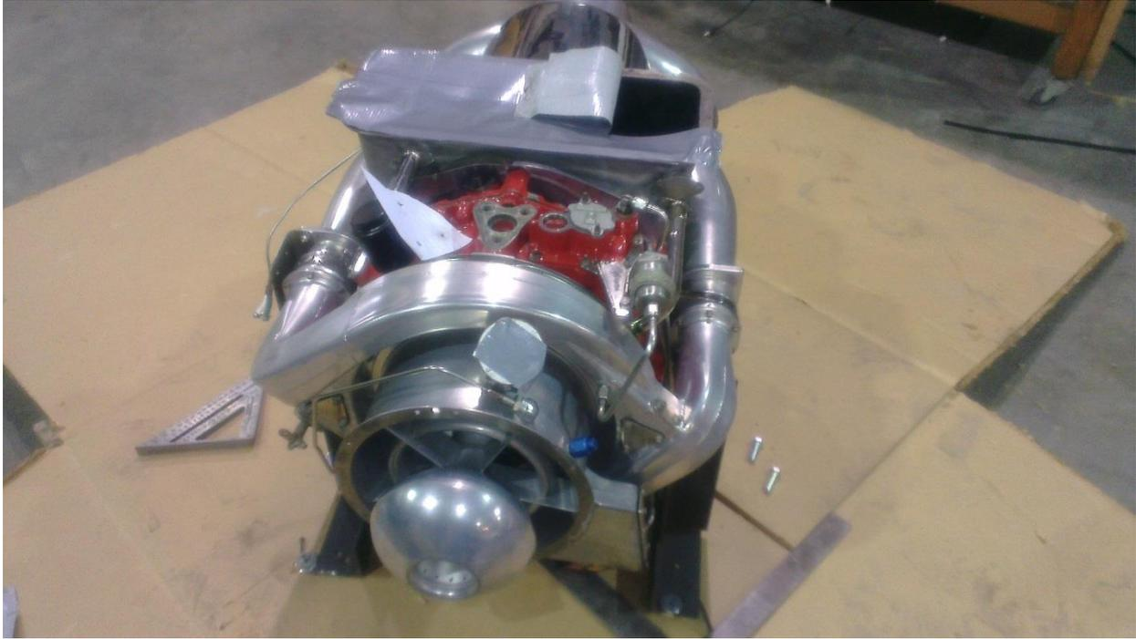
**Figure C-1 C28B Test Engine**
