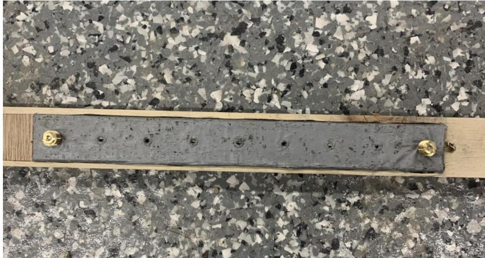
Figure 4 Steel spacer for brass inserts placed in mold slot
