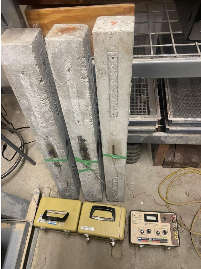
Figure 7. Control creep specimens connected to the P3500 strain indicator box
