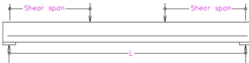
Figure 2.1 Traditional shear test set-up for concrete beams
