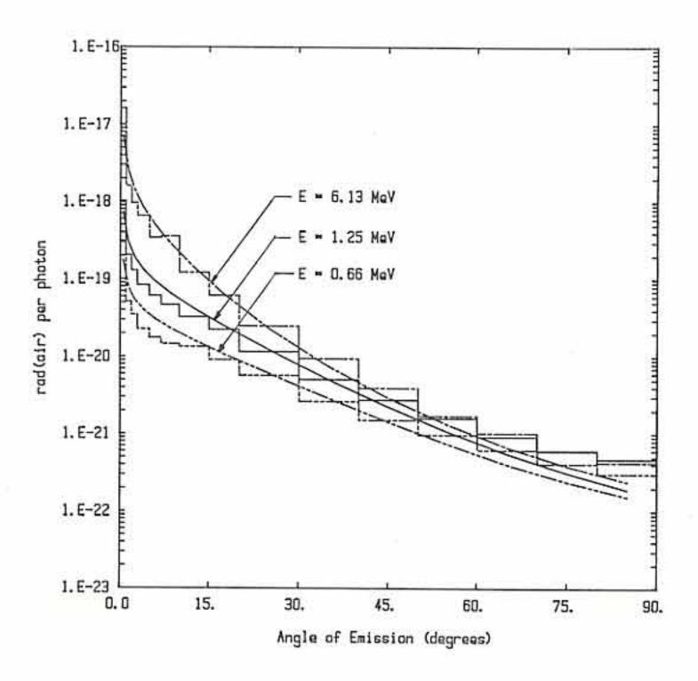
Fig. 4.1 Variation of the PRIGAM atmospheric scattering response function  $R(E,\phi,x)$  with angle of photon emission  $\phi$  at fixed source-detector distance x=500 m and at selected photon energies. Histogram: original RRA response functions based on Monte Carlo calculations [La79]. Lines: new response functions based on point-kernel calculations reported here.
