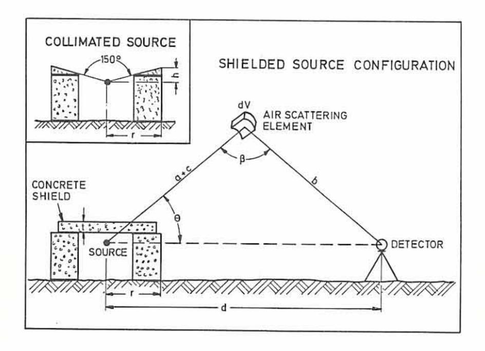
Fig. 4.9 Geometry for benchmark skyshine experiments. Source is in a concrete annular cylinder (2.5-m i.d., 4.35-m o.d., 2.29-m height) and either shielded from above by a concrete slab (21.0 or 42.8 cm thick) or collimated into a 150.5-degree vertical cone (inset). Distances a and b refer to the air path distances between the source and scattering element and between the scattering element and the detector respectively. Ray distance through concrete is denoted by c.
