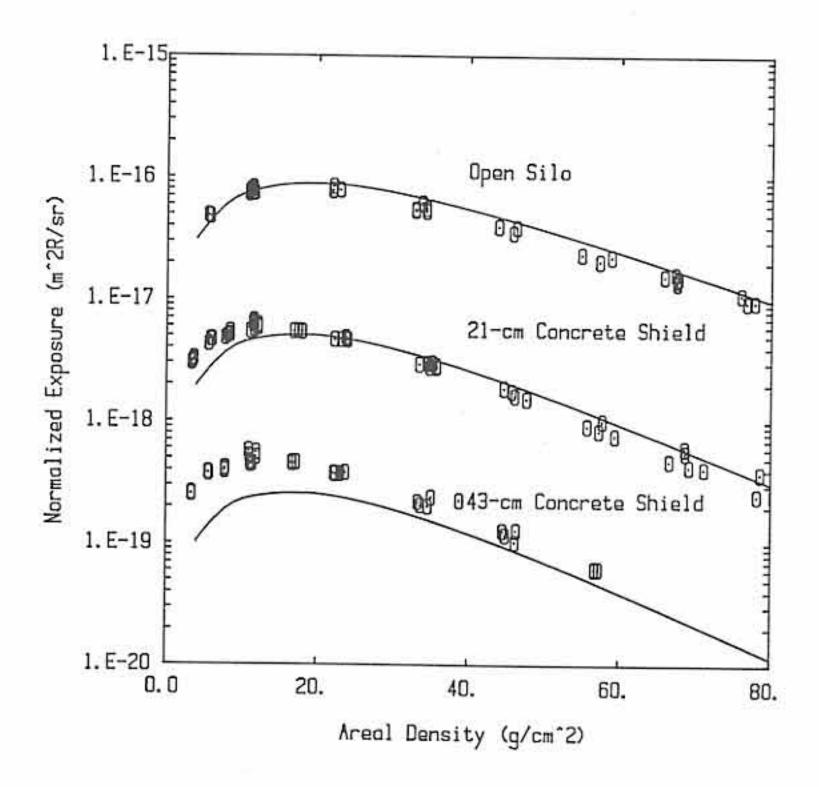
Fig. 4.10 Comparison of MicroShyshine results (solid lines) with experimental data for the conditions of the KSU benchmark skyshine experiments. A \*\*Co source is within a cylindrical silo with a 150.5-degree full-angle of collimation. Three cases are shown: (1) no overhead shielding, (2) 21 cm of overhead concrete shielding, and (3) 42.8 cm of overhead concrete shielding of density 2.32.g/cm<sup>3</sup>.
