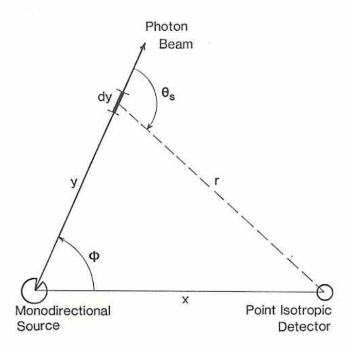
Fig. 3.1 Geometry for calculation of line-beam response functions.
