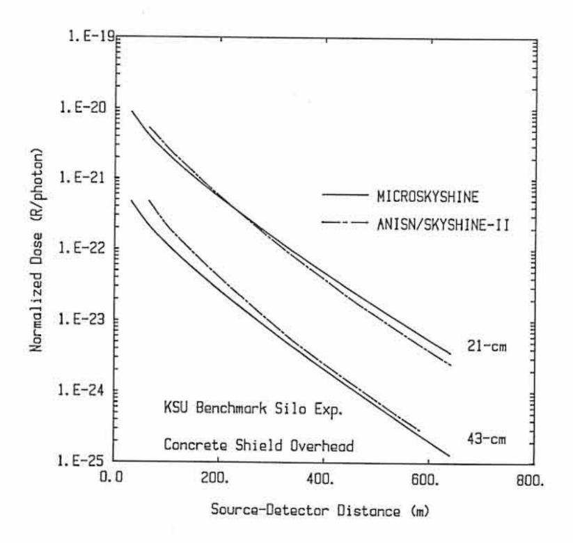
Fig. 4.11 Comparison of MicroSkyshine results (solid lines) with hybrid ANISN/SKYSHINE-II results [Ke82] (broken lines) for the conditions of the KSU benchmark skyshine experiments with overhead shielding.
