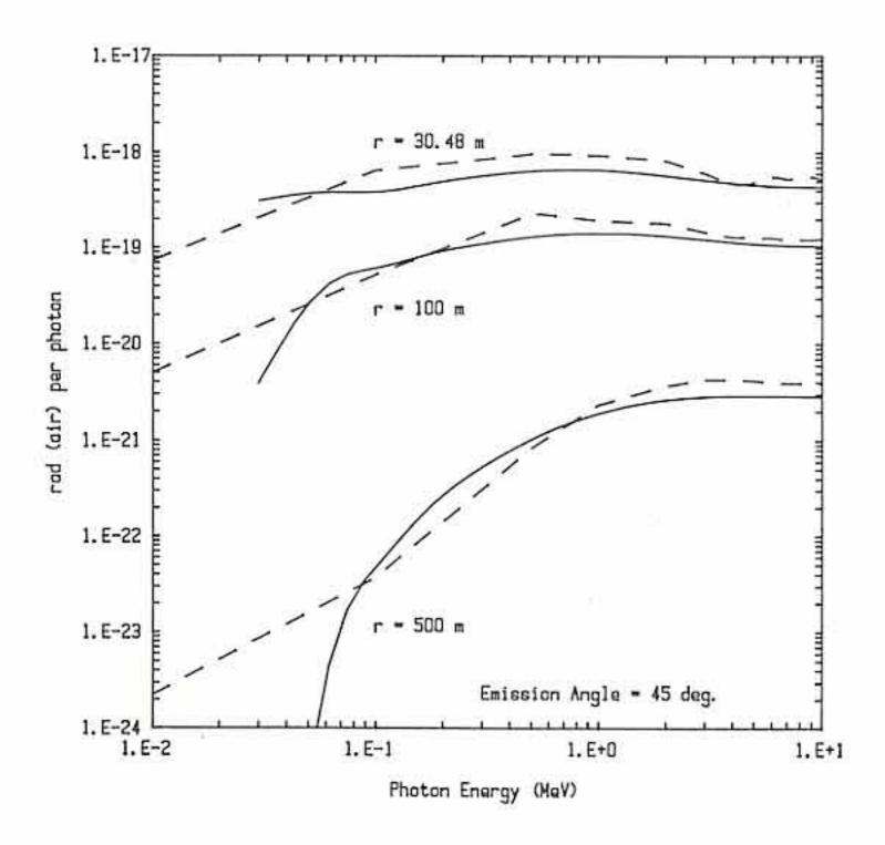
Fig. 4.2 Variation of the PRIGAM atmospheric scattering response function R(E,φ,x) with photon energy E at fixed angle of emission φ and at selected source-detector distances. Broken lines: original RRA response functions based on Monte Carlo calculations [La79]. Solid lines: new response functions based on point-kernel calculations reported here.
