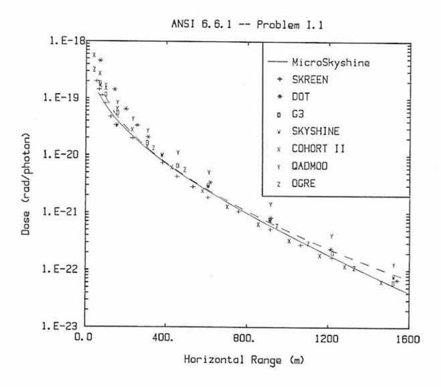
Fig. 4.7 Comparison of MicroSkyshine calculations with benchmark calculations for ANSI/ANS-6.6.1 Reference Problem I.1. Broken lines: MicroSkyshine calculations based on original RRA response functions [La79]. Solid lines: MicroSkyshine calculations based on new point-kernel response functions reported here.
