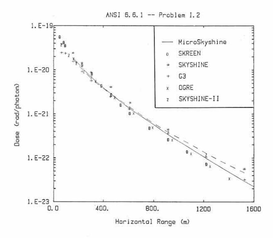
Fig. 4.8 Comparison of MicroSkyshine calculations with benchmark calculations for ANSI/ANS-6.6.1 Reference Problem I.2. Broken lines: MicroSkyshine calculations based on original RRA response functions [La79]. Solid lines: MicroSkyshine calculations based on new point-kernel response functions reported here.
