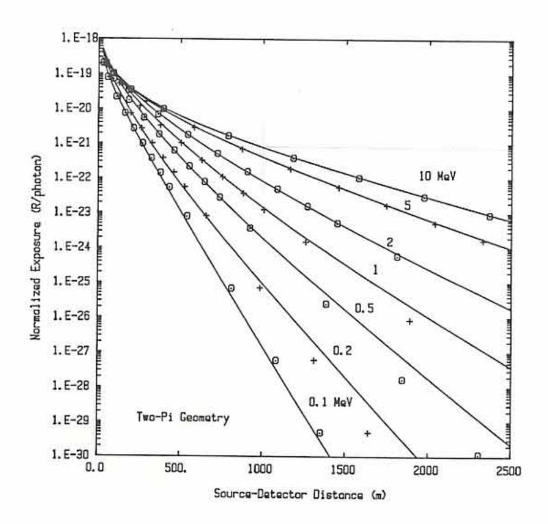
Fig. 4.4 Comparison of MicroSkyshine results (solid lines) with moments-method results (data points) for the scatteredradiation dose arising from a point source emitting photons only in the 2π-steradian upward hemisphere of directions in an infinite atmosphere.
