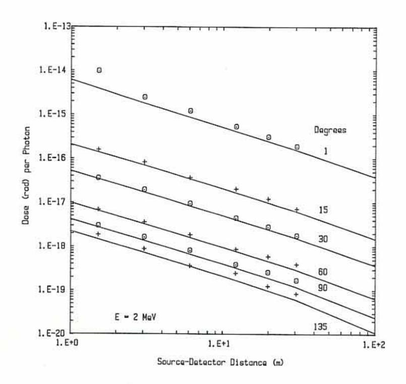
Fig. 4.3 Comparison of new PRIGAM atmospheric scattering response functions (solid lines) with response functions calculated by Lynch, et al. [Ly58] for 2-MeV photons at selected angles of emission.
