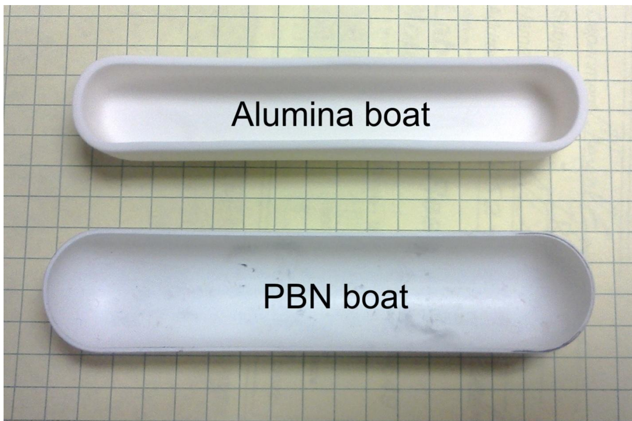
Figure 2-7: Photograph of the alumina and pBN sample boats used for crystal growth (each square is 0.25" x 0.25").
