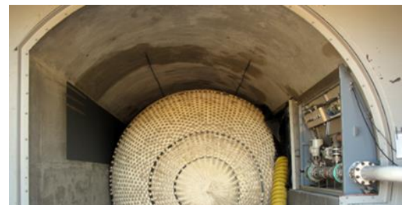
Figure 22: Testing the resilient tunnel plug
