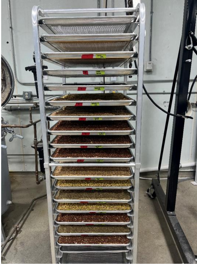
Figure 4-2 Commercial baking rack with baking pans that seeds were placed on to germinate
