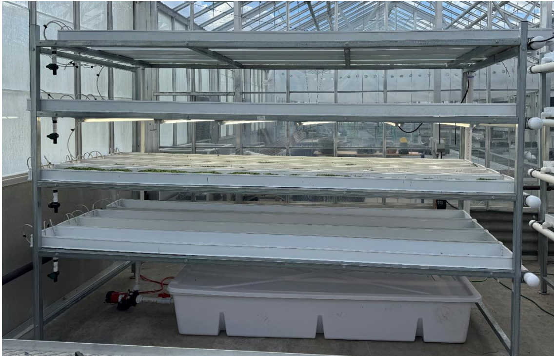
Figure 5-1 Commercial microgreen tower used for production of sorghum sprouts and sorghum microgreen in larger quantities. Tower contains four levels with four trays each, 6 lights on each level, and each tray has 2 waterers.
