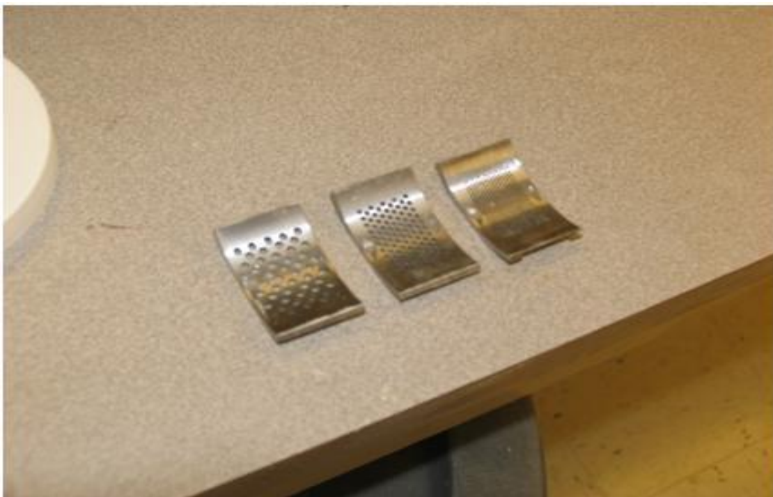
Figure A-3: Photo of Hammer Mill Screen Sizes, 3.0 mm, 2.0 mm, and 1.0 mm from Left to Right
