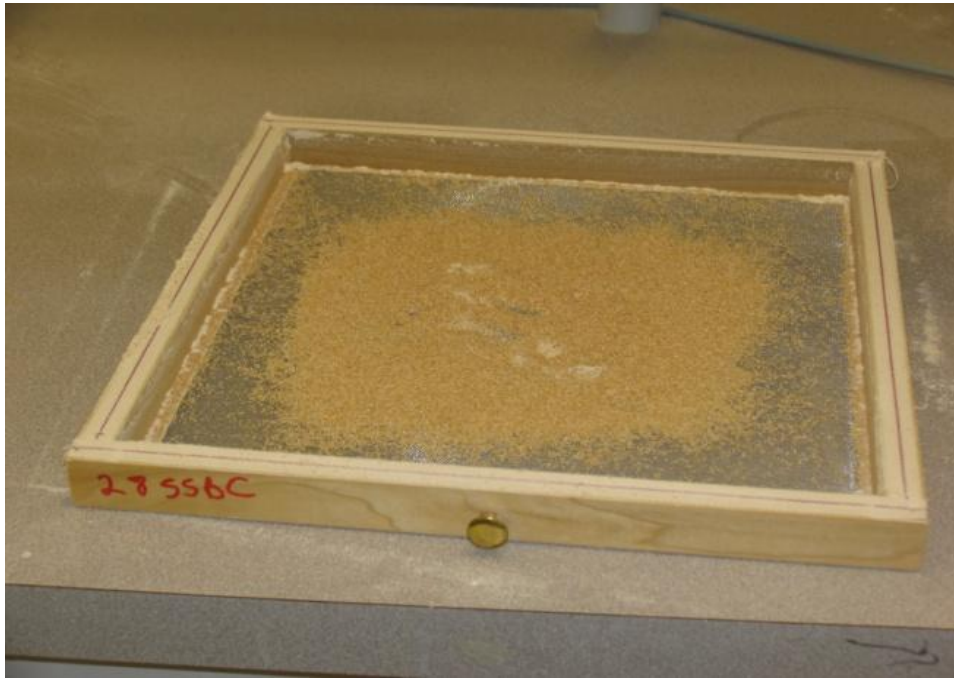
Figure A-8: Photo of 28 Stainless Steel Bolting Cloth, Medium Stock
