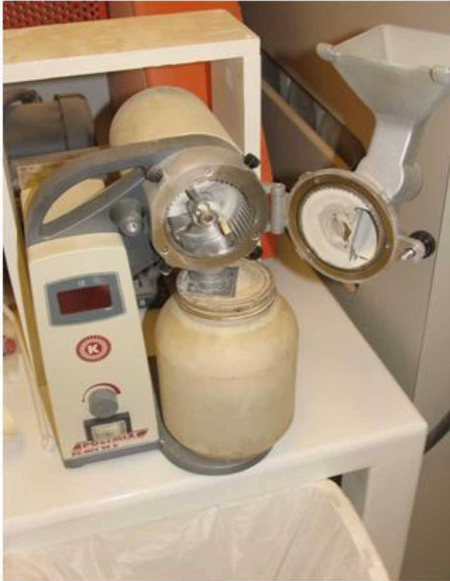
Figure A-1: Photo of Experimental Hammer Mill Used for Initial Grinding
