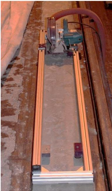
(a) Track-mounted saw used to cut groove
