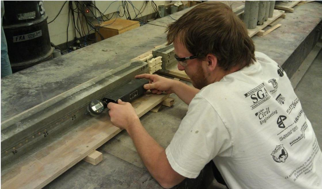
Figure 31 Surface distance measurement though Whittemore gage
