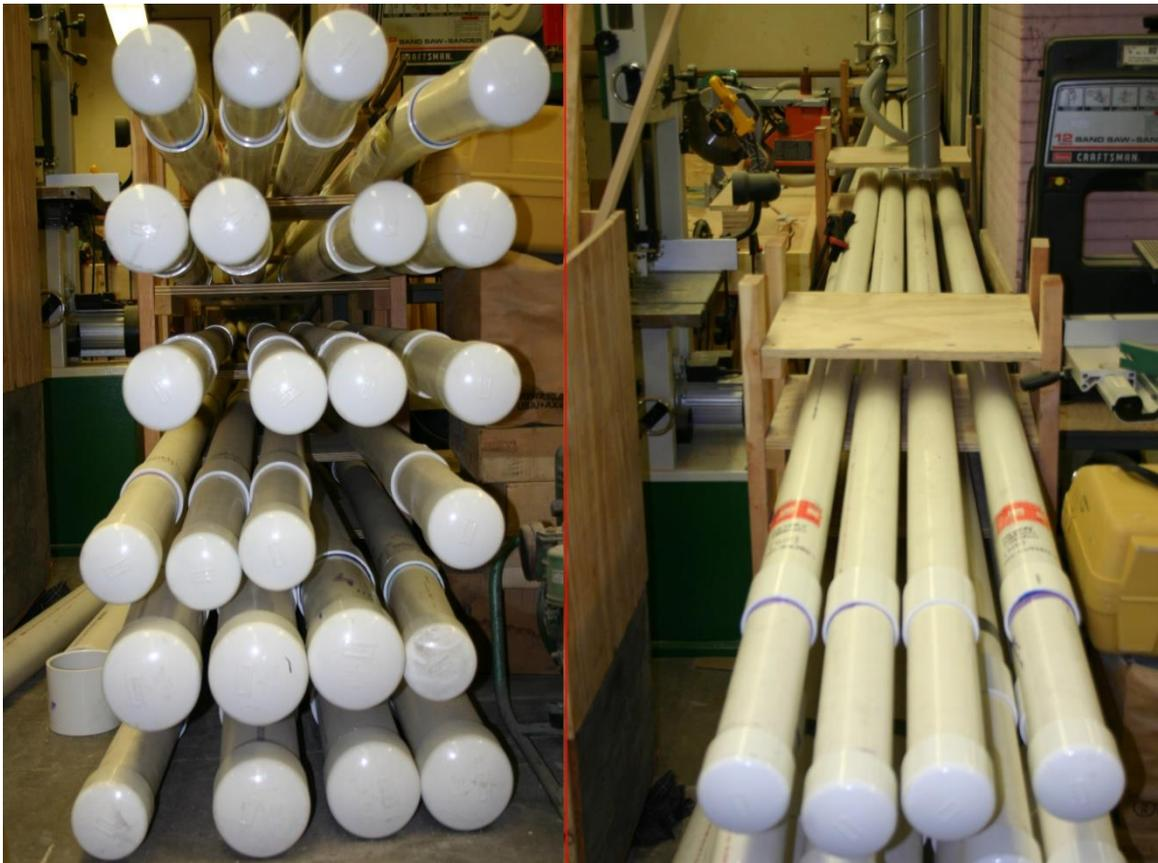
Figure 8 Preservation of reinforcement at KSU laboratories (Arnold, 2013)
