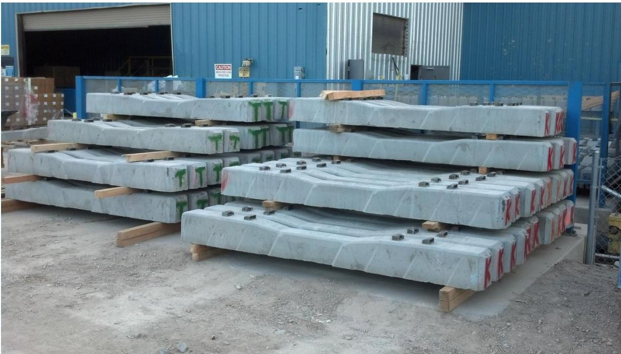
Figure 101 Separation of in-track loading ties (“T”) and KSU ties (“K”) during Plant-Phase
