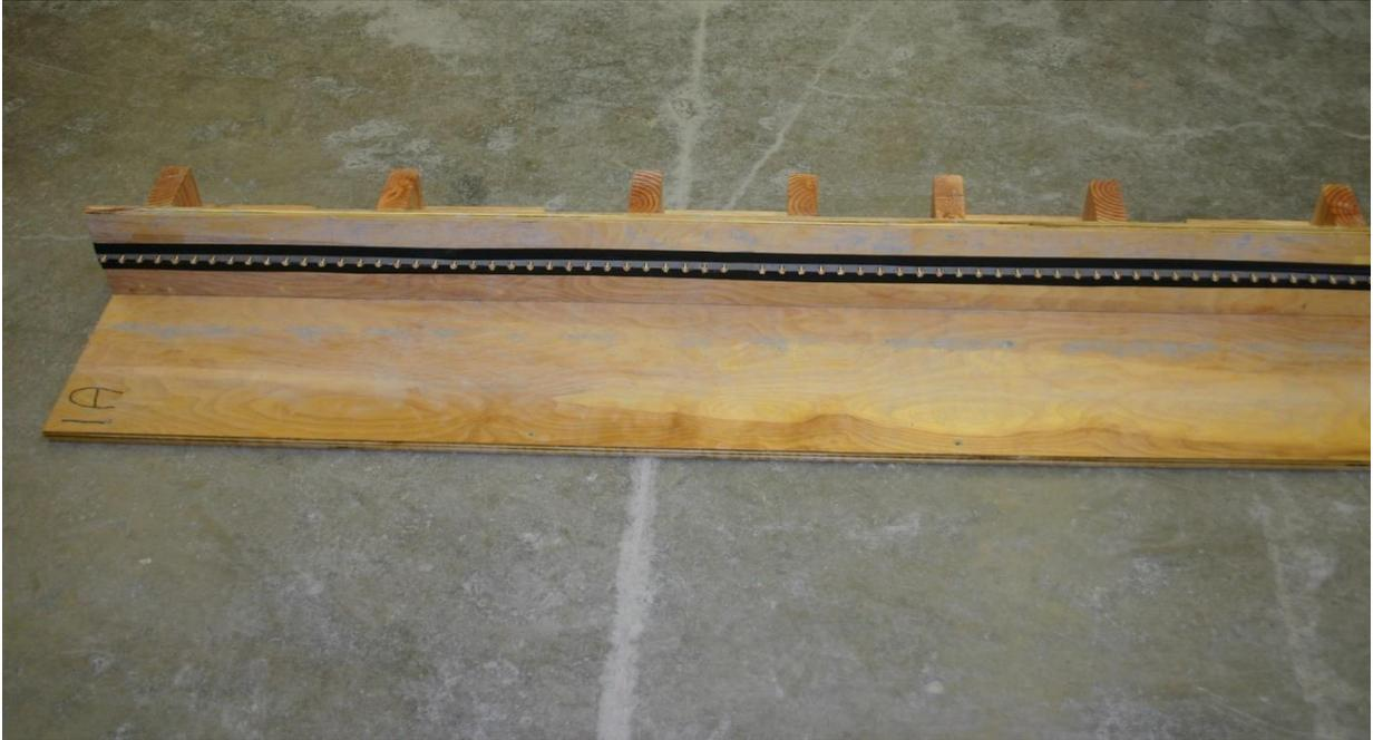
Figure 22 Wooden side form equipped with brass inserts before casting
