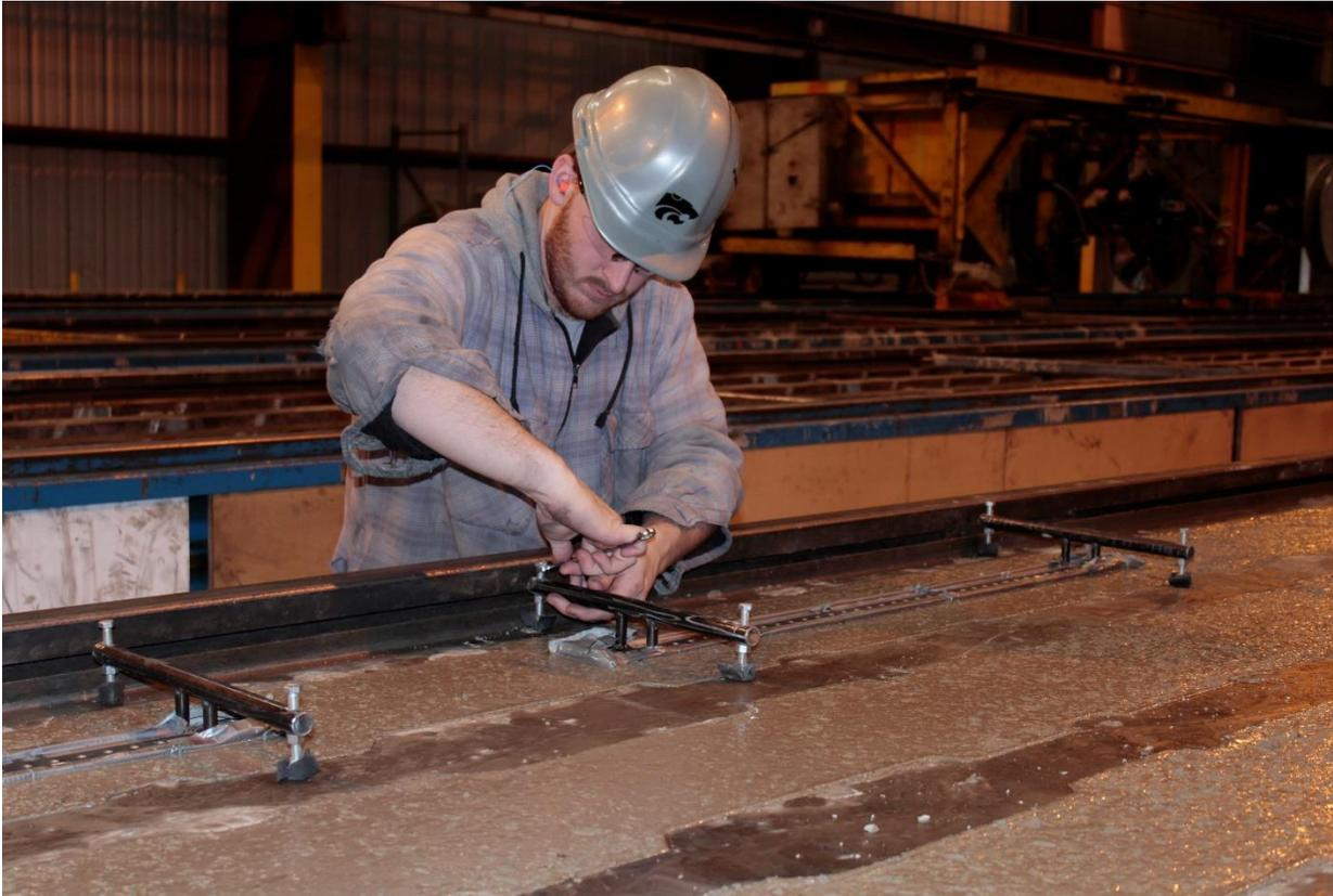
Figure 94 Steel bars used to hold brass inserts at proper spacing in the concrete cross-ties
