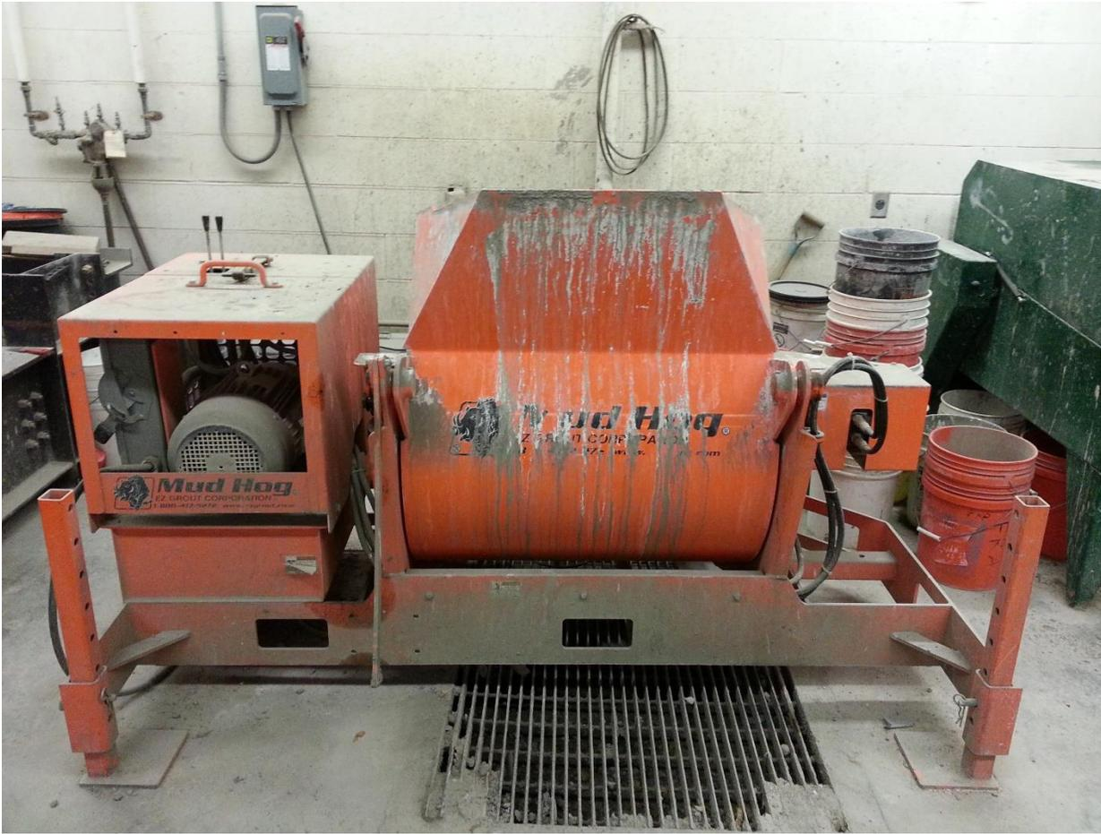
Figure 13 Concrete Mixer used during the Lab-Phase
