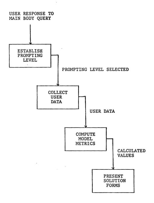
Figure 1. General Logic Flow of the Main Program.
