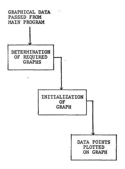
Figure 2. General Logic Flow of Display Driver Program.
