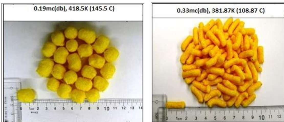
Figure 3-5 Scale comparison of the expansion for product with highest sectional expansion and lowest sectional expansion.
