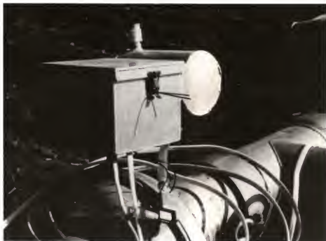
Figure 4. Solenoid Valve Connected in Diaphragm Line.
