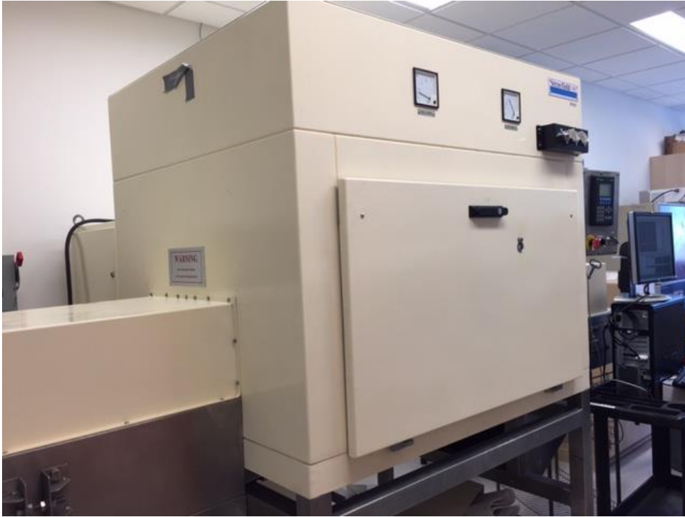
Figure 3-1. Radio frequency dielectric heating unit (Strayfield Limited, Theale, Berkshire, England) at University of Nebraska-Lincoln.
