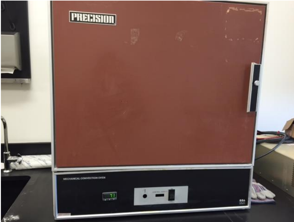
Figure 3-5. The convection oven (Thelco, GCA/Precision Scientific, Schaar Scientific Company, Chicago, IL) used to hold nonfat dry milk for designated times at University of Nebraska - Lincoln.
