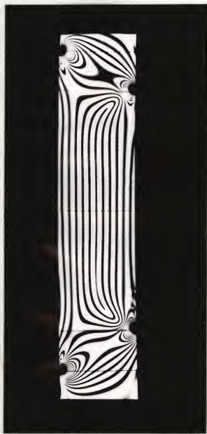
Fig. 5. Dark field photograph of isochromatics for pure bending.
