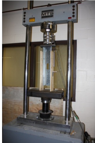
Figure B. MTS Testing Machine and specimen
