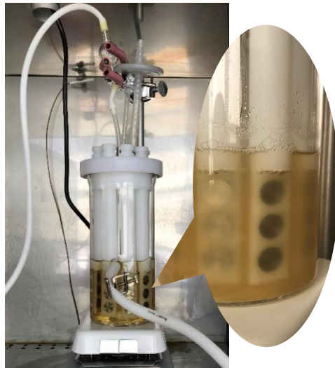
Figure 3.1. CDC Biofilm Reactor ® used in this study to grow multi-strain L. monocytogenes biofilms under high shear conditions (coupons were zoomed in).
