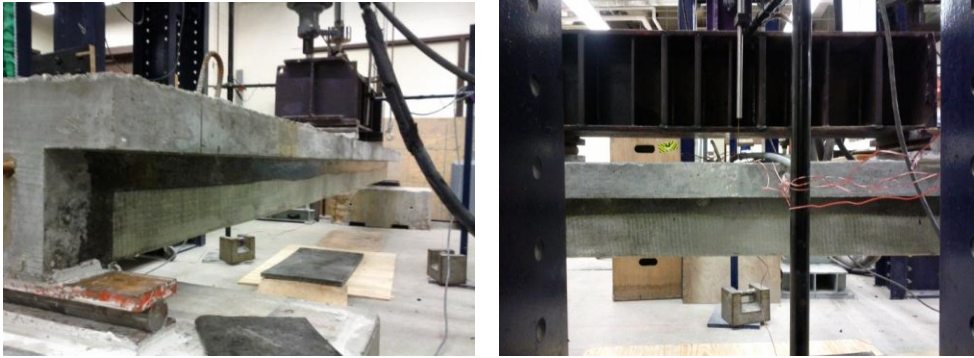
Figure 3-28: Two LVDTs Are Used For Recording the Deflection in Both Sides of the Beam Midspan.
