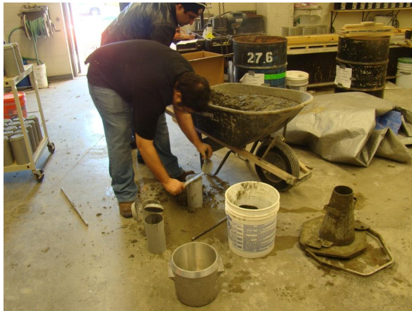
Figure 3-1: Casting of Concrete Cylinders.
