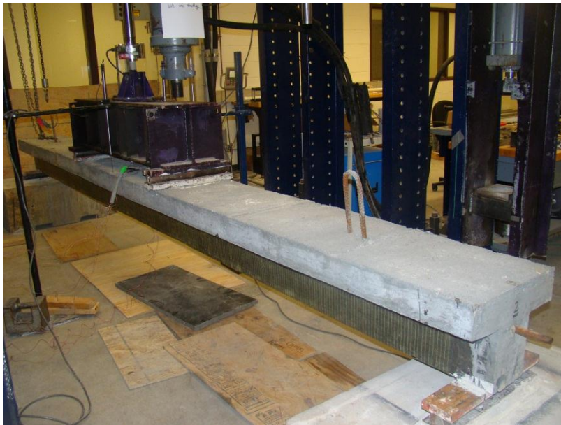
Figure 4-7: Beam T2 with Full Length of NSM Bars before Testing.
