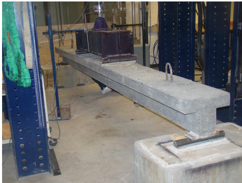
Figure 4-1: Control Beam T1 before Testing.
