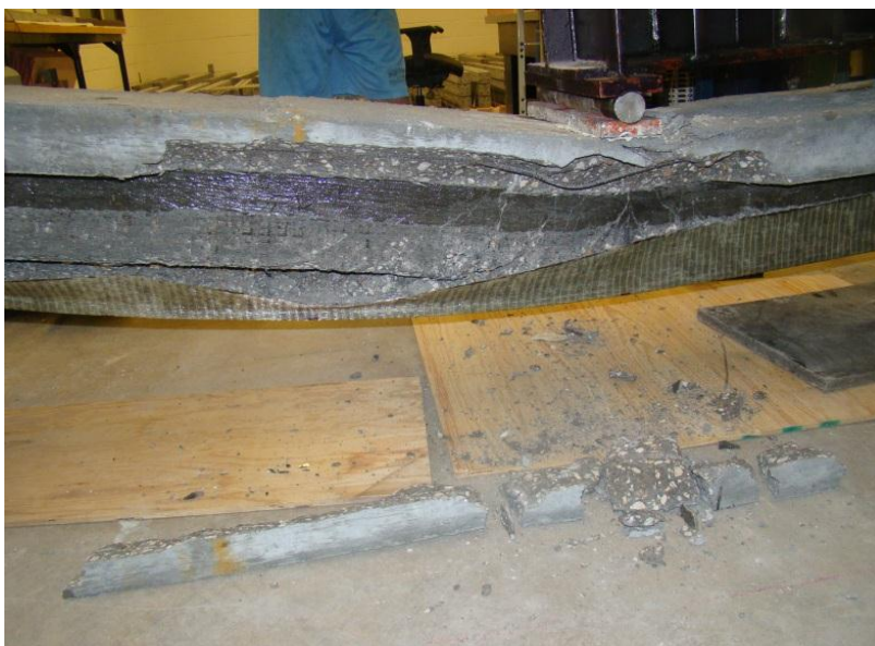
Figure 4-8: Cover Delamination Failure followed by GFRP Debonding.
