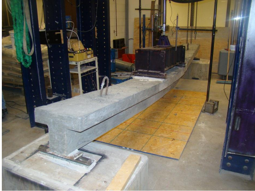
Figure 4-2: Beam T1 Just Prior to Failure.
