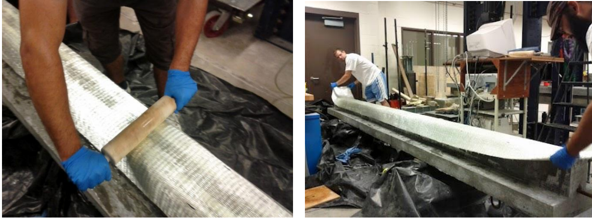
Figure 3-23: Installing the FRP Sheets.
