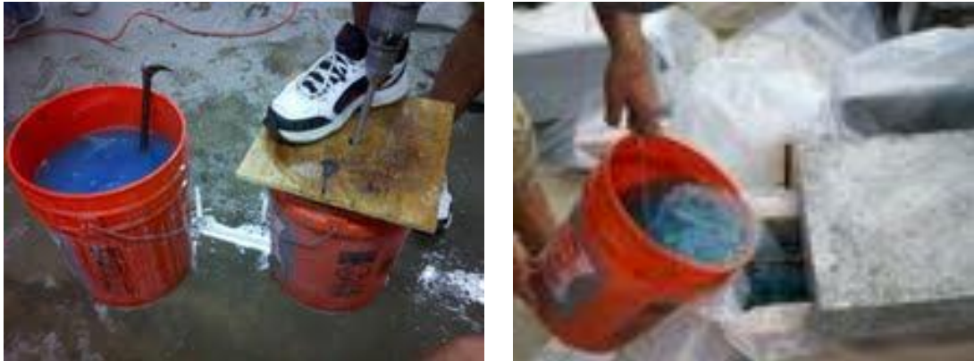
Figure 3-25: Dissolving Deicing Salt in Tap Water.
