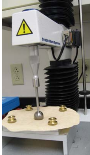
Figure 4. Stretchability/Flexability test for flour tortillas
