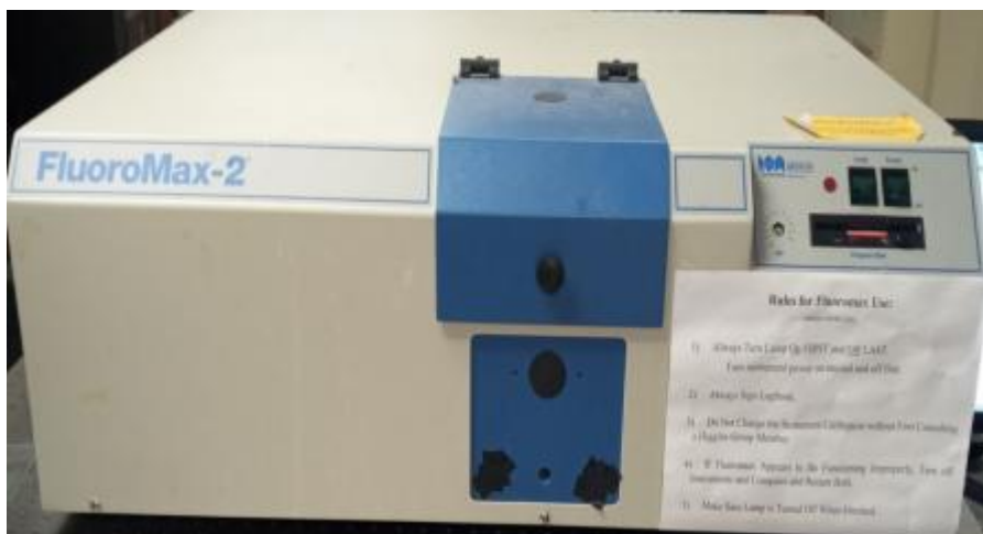
Figure 2.4. Spectrofluorometer (FluoroMax-2) photo by Samson Adegbite.
