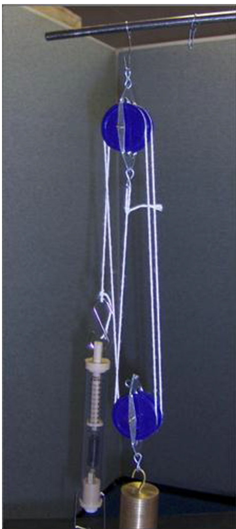
FIG. 2 (color online). The physical manipulatives for the pulley experiment included pulleys, string, a spring scale, a meter stick, and a mass.
