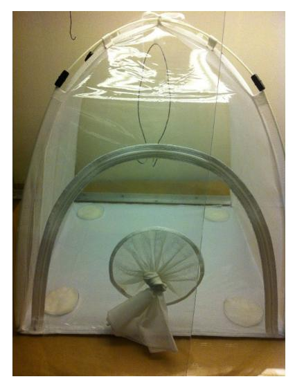
Figure 3.3. BugDorm rearing cage used for the oviposition experiments.
