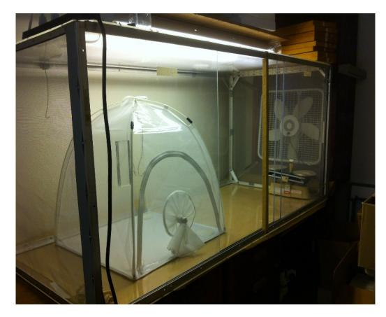
Figure 3.4. BugDorm rearing cage placed in a wind tunnel for the oviposition experiments.
