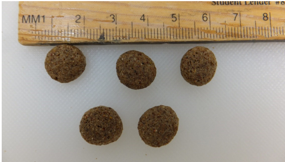
Figure 4-3. Mill-feed sample (MF) composed of bran, shorts (finer bran), red dog (leftovers of the last flour cloth in the mill) and some coarse flour.
