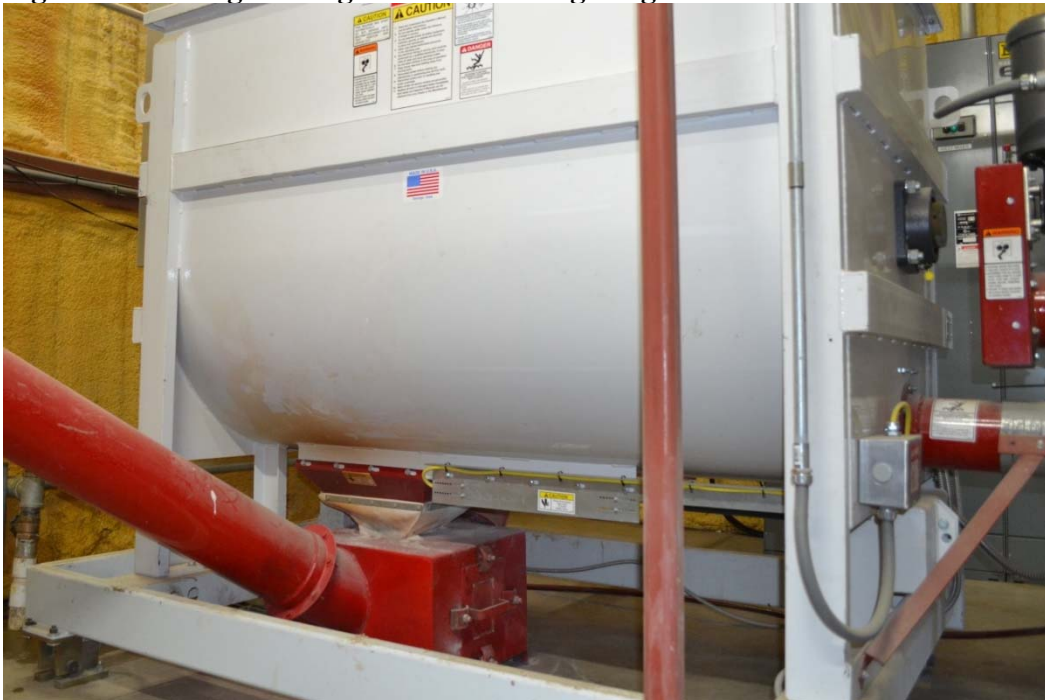
Figure 1.7 Mixing/holding bin and discharge auger
