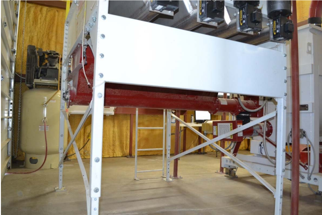
Figure 1.6 Underneath Mini-bins load cells and auger system
