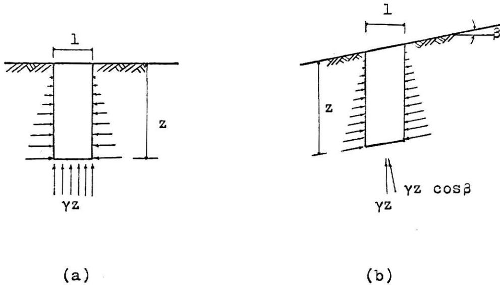
Fig. (1) (a) The vertical stress at depth  $z$  caused by the self-weight of soil with horizontal surface
