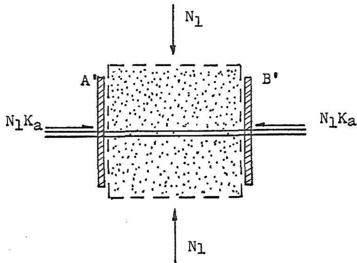
Fig. (8-b) A cube of reinforced earth is in equilibrium
