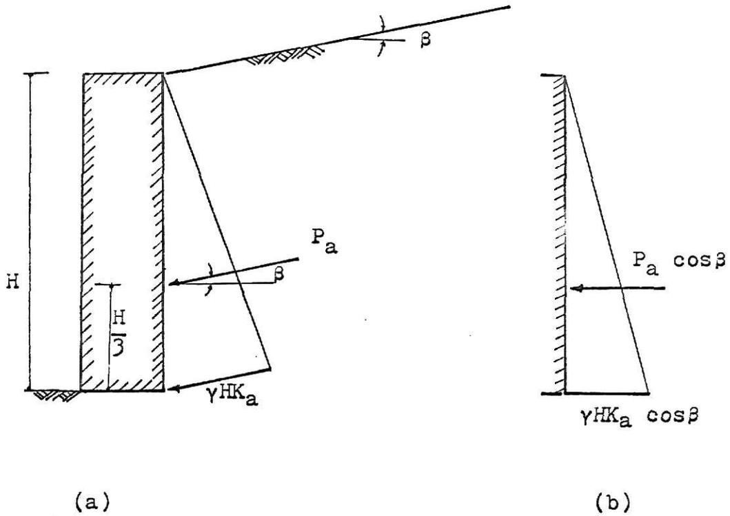
Fig. (9) (a) Active earth pressure diagram
