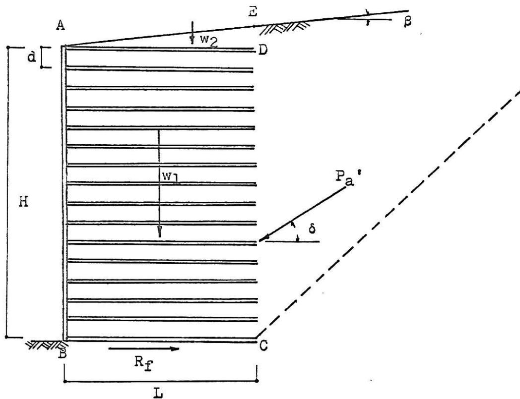
Fig. (11) Forces acting on a strap reinforced earth retaining wall
