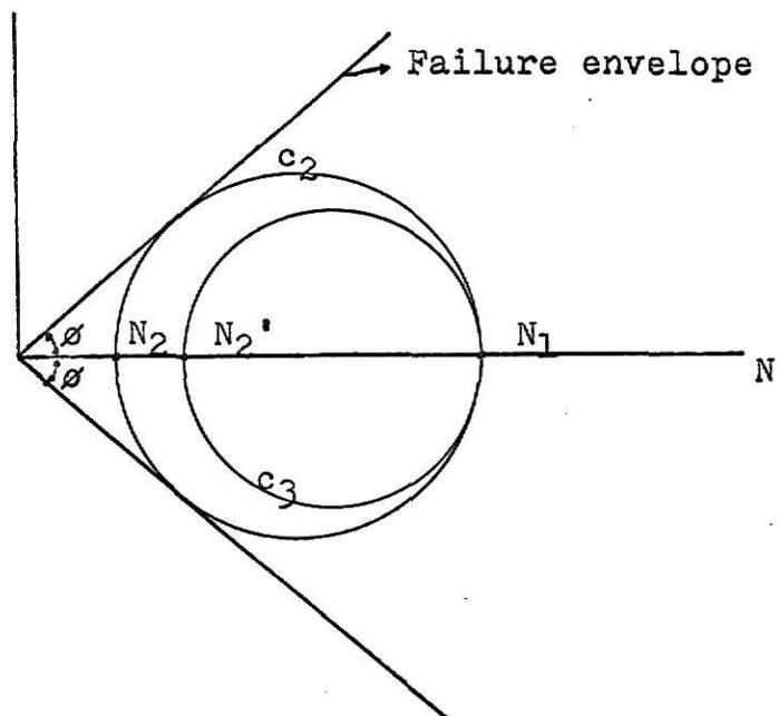
Fig. (7-b) Graphic representation of state of the stress at failure,  $c_2$  represents the earth in elastic equilibrium
