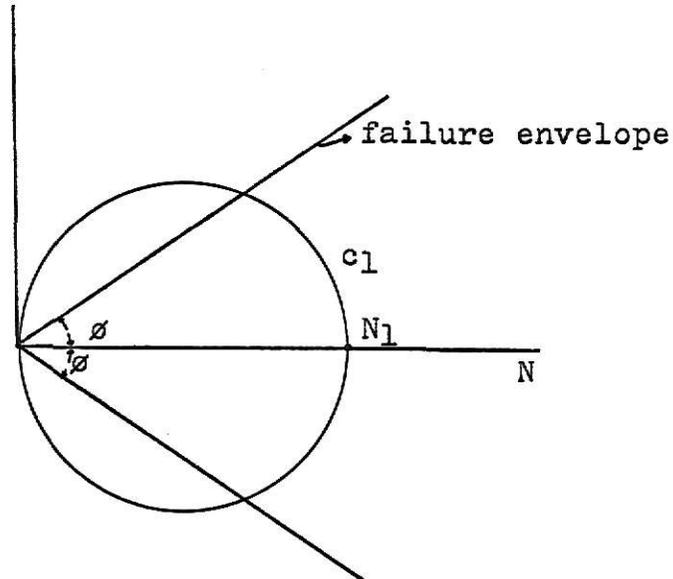
Fig. (6-b) Mohr's circle represents the state of the stress in the unbounded earth
