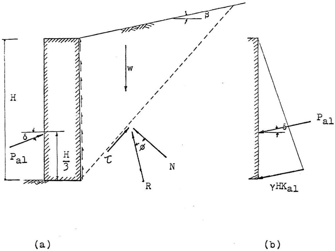
Fig. (3) (a) Failure wedge and acting forces for active earth pressure with the wall friction considered
