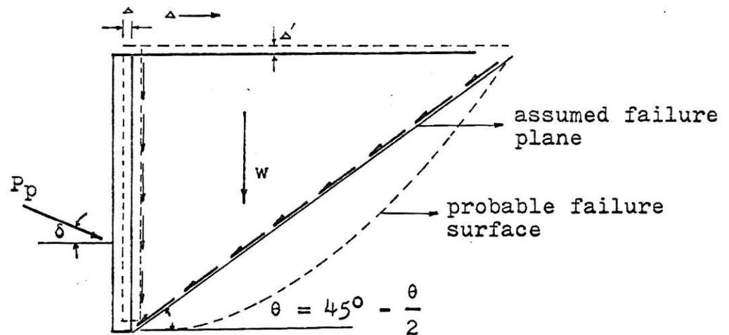
Fig. (2-b) Wall movement to develop passive pressure
