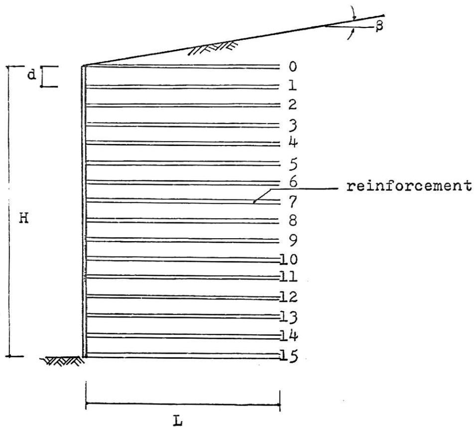
Fig. (10) A retaining wall constructed of strap reinforced earth
