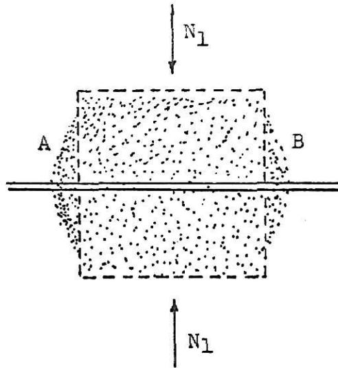
Fig. (8-a) A reinforcement is introduced horizontally into the cube of non-cohesive earth which is subjected to a vertical compressive force  $N_1$
