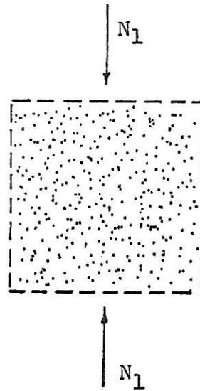
Fig. (6-a) A cube of non-cohesion earth is subjected to a compressive force  $N_1$  on its two faces
