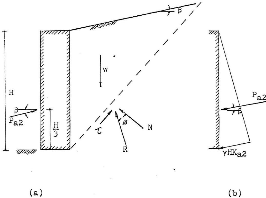
Fig. (4) (a) Failure wedge and acting forces for active earth pressure with the wall friction neglected
