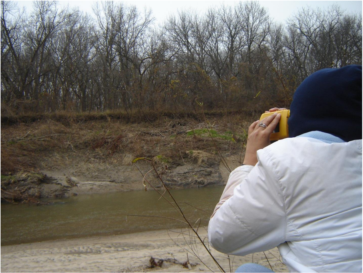
Figure A.4 Measuring the active channel width (ACW) using the LaserAce™ instrument.
