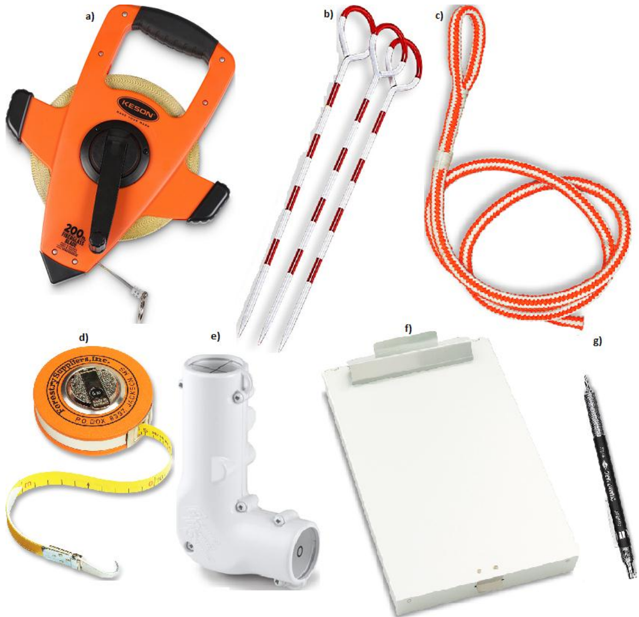
Figure A.3 Equipment used in data collection: a) Reel fiberglass tape, b) Chaining pins, c) Ropes, d) Diameter tape, e) GRS densitometer, f) Sheet holder, g) Pencil.
