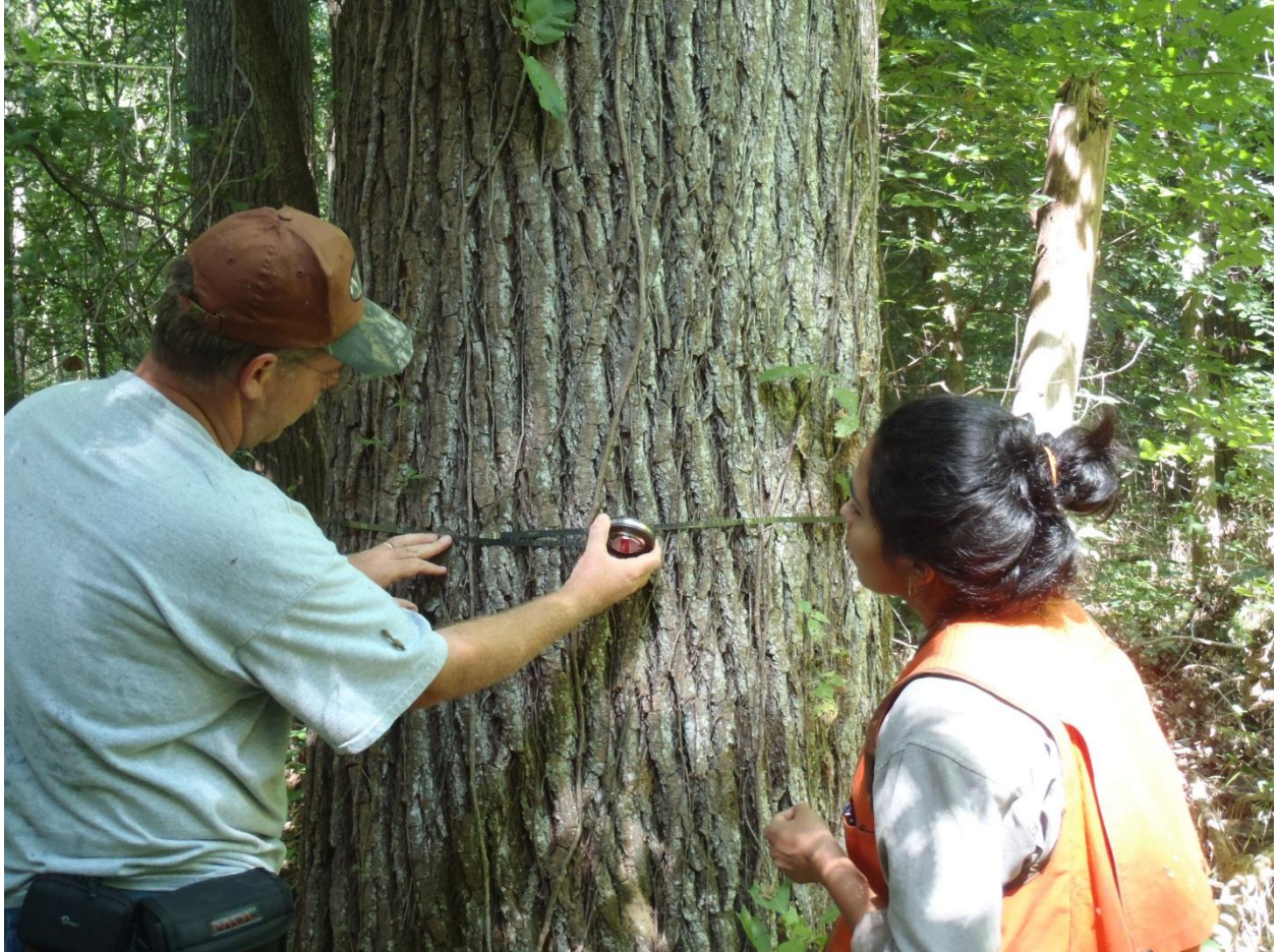
Figure A.6 Measuring the diameter at breast height (dbh) with a diameter tape instrument.
