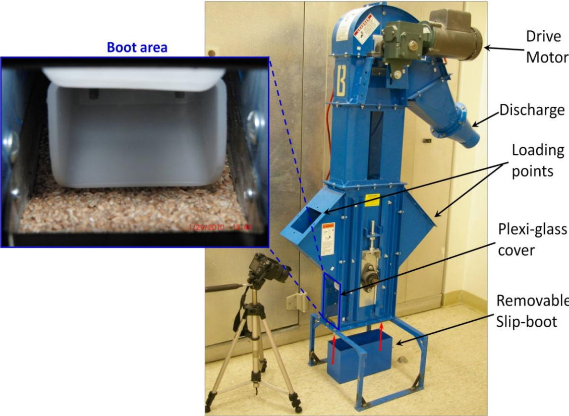
Figure 2.1. Pilot-scale bucket elevator leg boot arrangement.
