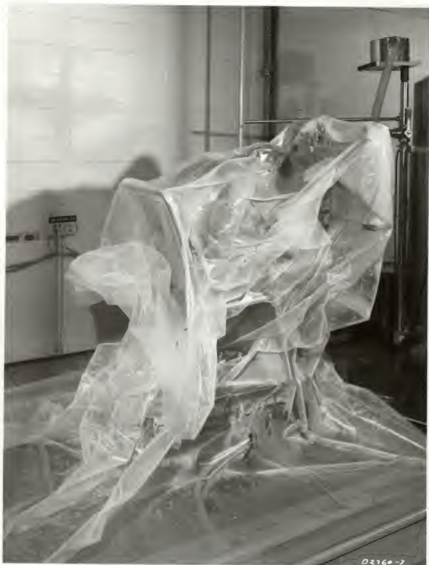
Figure 4. Polyethylene Test Cell Collapsed Showing the Degree of Evacuation of Air From the Test Cell
