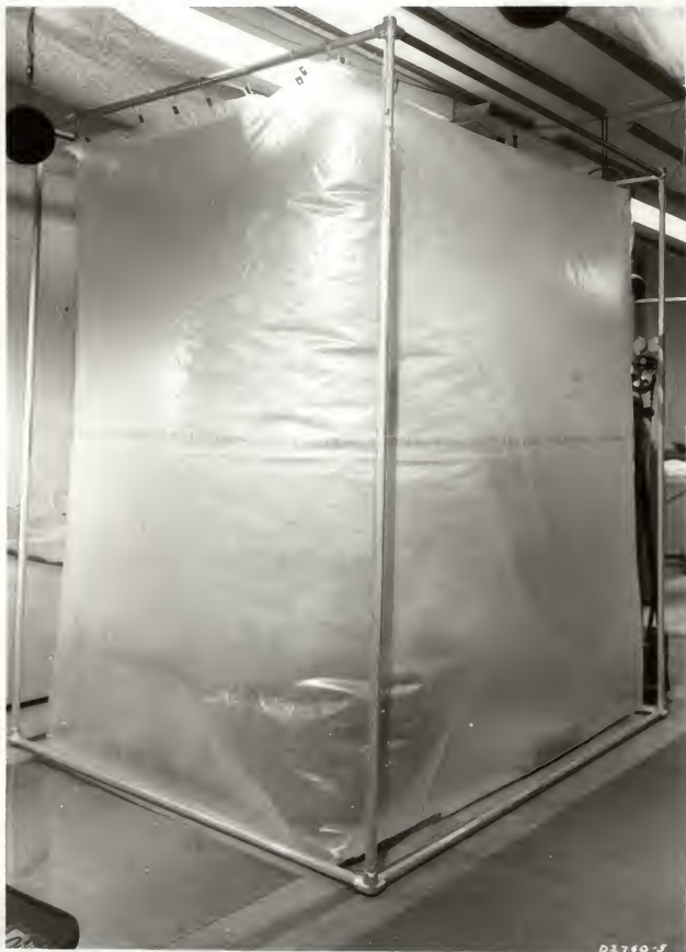
Figure 1. Inflated Polyethylene Test Cell Supporting Structure
