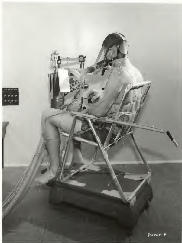
Figure 2. Subject Seated in Test Configuration Showing the Mask, Valve Humidity Sensor, Scale, and Thermister Junction Board, Test Cell Removed.
