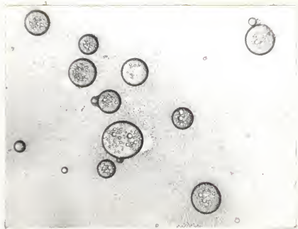
Fig. 7. Appearance of starch-chloral hydrate-furfural coacervate drops showing vacuolation and very small droplets formed as a result of electrophoresis. Mag. 300X
