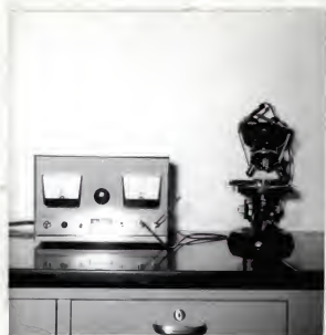
Fig. 2. Modified apparatus of Bungenberg de Jong and power supply used in electrophoresis of starch coacervates showing details of construction.
