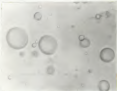
Fig. 9. Starch-chloral hydrate-gelatin coacervate drops showing demixing of the components of the coacervate induced by electrophoresis. Gelatin has accumulated in the dark outer area of the drop and the light inner area of the drop consists of starch-chloral hydrate. Mag. 300X
