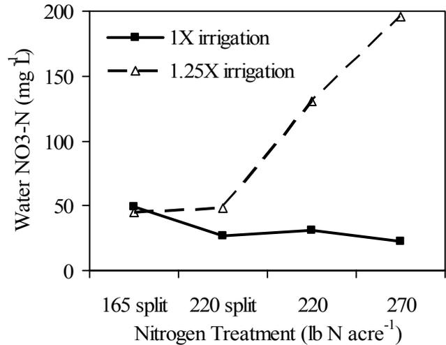
Figure 3. Water NO<sub>3</sub>-N concentration at the 60-inch depth on July 23, 2002 at Ellinwood. The irrigation by N treatment interaction was significant.
