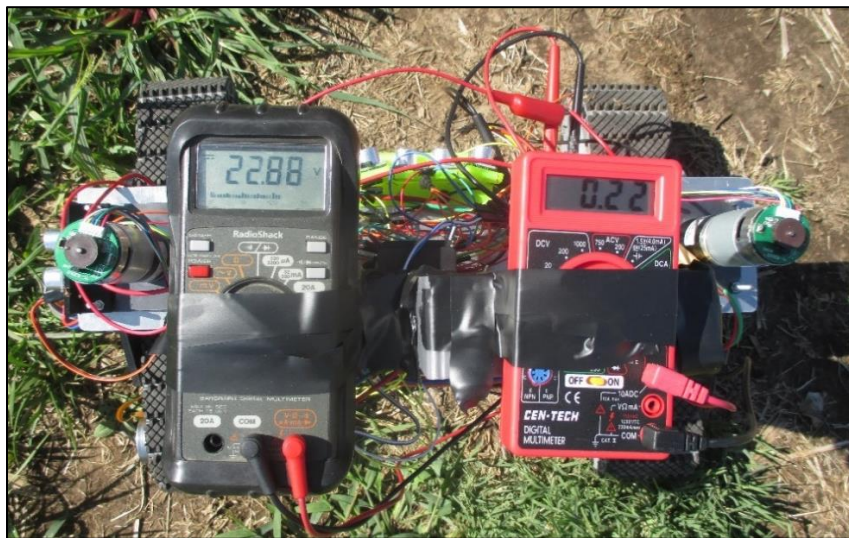
Figure 38 - Measuring Power Consumption. Left-Voltmeter, Right-Ammeter
