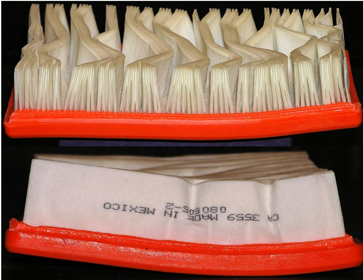
Figure 4.11: Top and side view of an air filter after contact with foam. The bottom image shows the deformation of a full-sized Fram™ air filter resulting from foam ingestion.
