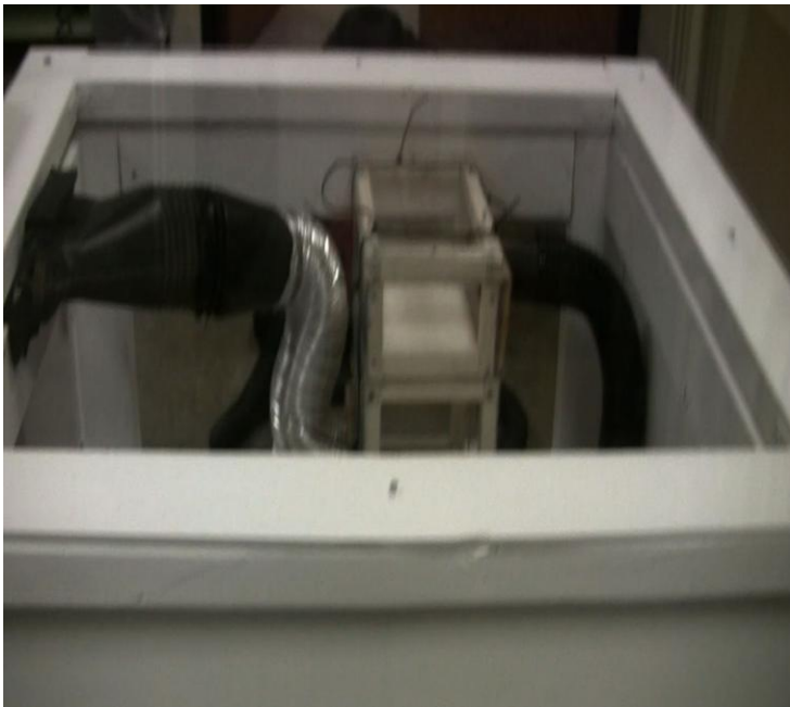
Figure 4.18: Half scale model of the induction system apparatus without pressure sensors.
