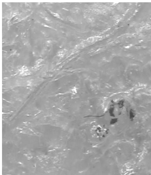
Figure 2.6: Surface of filter medium after contact with foam
