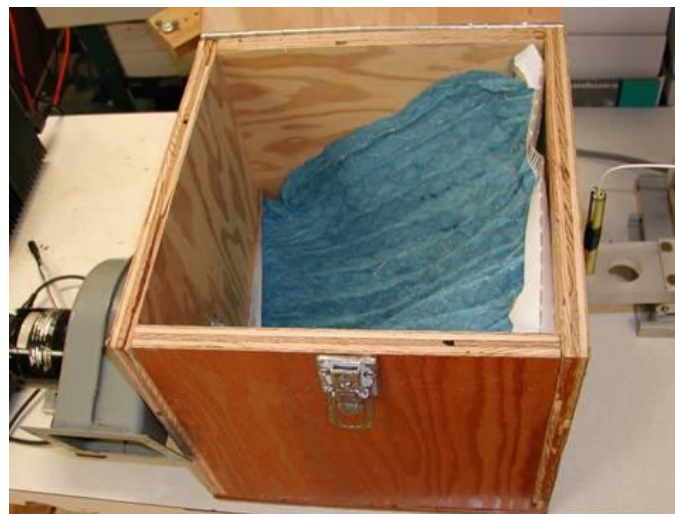
Figure 4.4: Addition of an air filter improved the velocity distribution.
