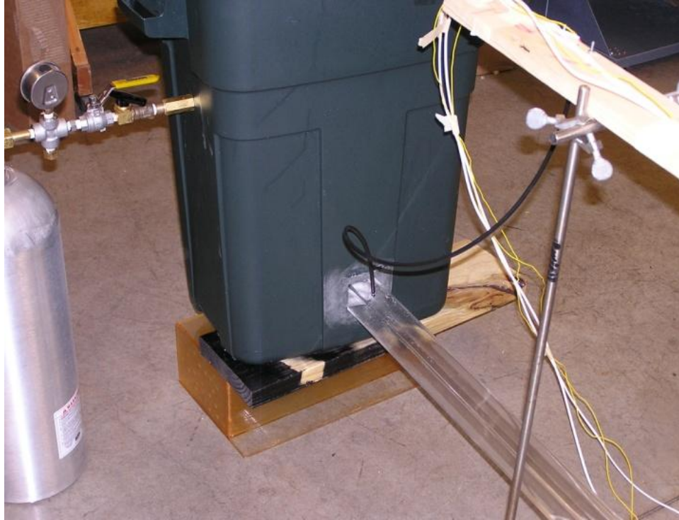
Figure 4.7: Apparatus for evaluating foam deformation and flow in a square (4.35 by 4.35 cm) acrylic plastic duct
