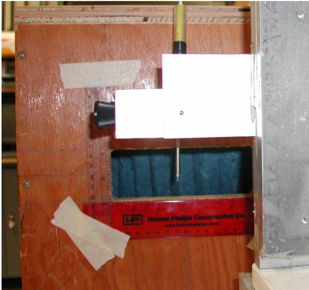
Figure 4.3: The air induction port and hot wire anemometer in position.
