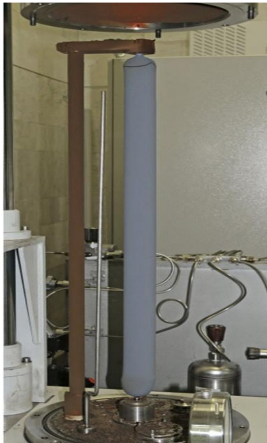
Figure 1: Polycrystalline ^{28}\text{Si} ingot in a deposition apparatus 8
