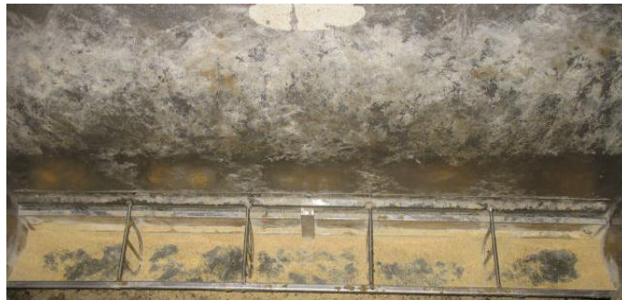
Figure 3-10. Conventional dry feeder with a 2.11- to 2.84-cm opening (setting 8) and \approx 57\% trough coverage.
