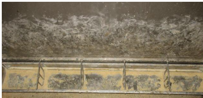
Figure 3-7. Conventional dry feeder with a 2.03- to 2.72-cm opening (setting 8) and \approx 21\% trough coverage.
