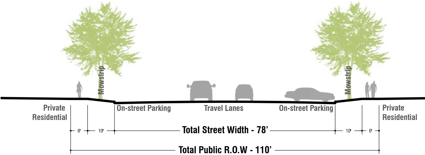
Figure 7.18 Typical main street sections - Selden (Scale: 1" = 20')
