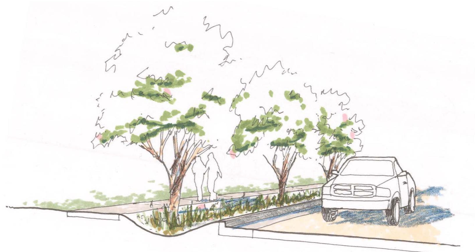
Figure 5.16 Street-side bioswale detailed section
